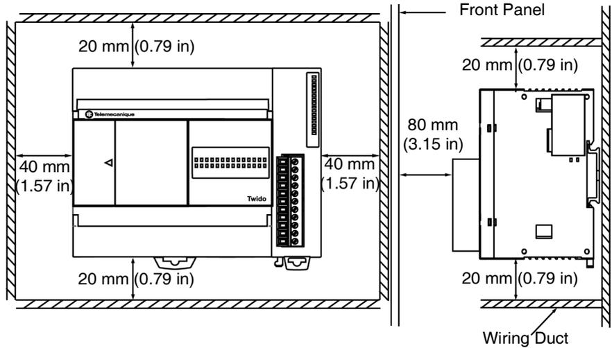
**Minimum Clearances for a Modular Base and Expansion I/O Modules**
