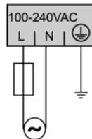
**DC Power Supply Wiring Schematic**
