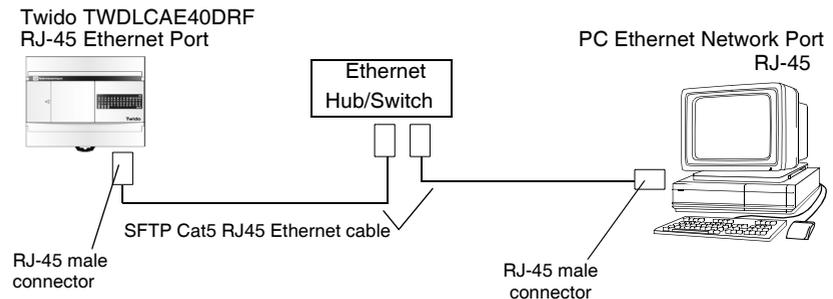
**Note:** The PC running the TwidoSuite application must be Ethernet-capable.
