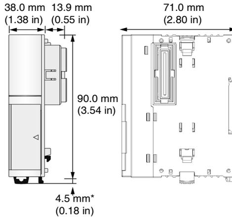
**Second Serial Interface Expansion Module with Operator Display Dimensions**
