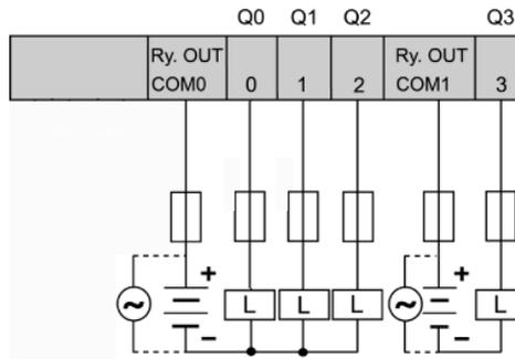
This schematic is for the TWDLC•A16DRF series bases.
