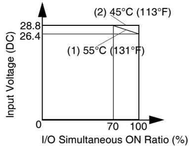
Also, when using the above-mentioned bases at 45°C (113°F), all I/O can be turned on simultaneously at input voltage 28.8 VDC as indicated with line (2).
