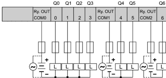
This schematic is for the TWDLC•A24DRF series bases.
