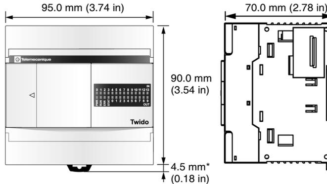
**TWDLCA•40-DRF** The following diagrams show the dimensions for the TWDLCA•40DRF series Compact base.
