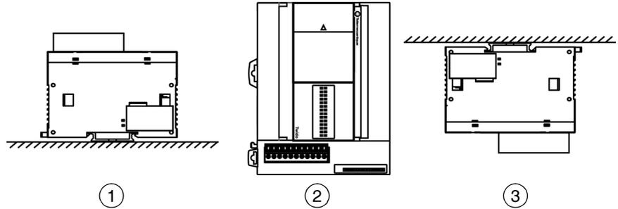
**Incorrect Mounting Positions for Modular Bases**
