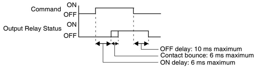
**Transistor Source Output Contact**
