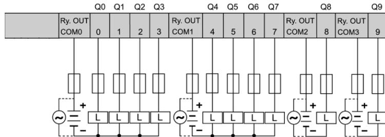
This schematic is for the TWDLCA•40DRF series bases.
