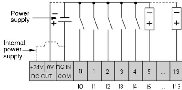
The following DC source input wiring schematic is for the TWDLCA•40DRF series bases.
