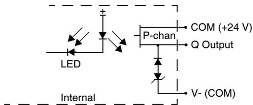
**Transistor Sink Output Contact**
