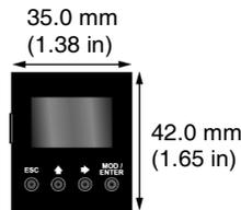
**Operator Display Module Specifications**
