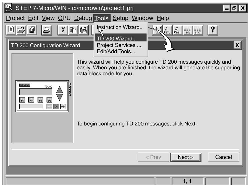
Figure 5-3 Accessing the TD 200 Configuration Wizard
