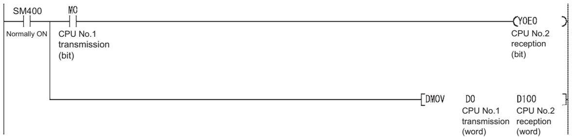
Diagram 8.13 Program example for sending bit and word data from CPU No. 1 to CPU No. 2
