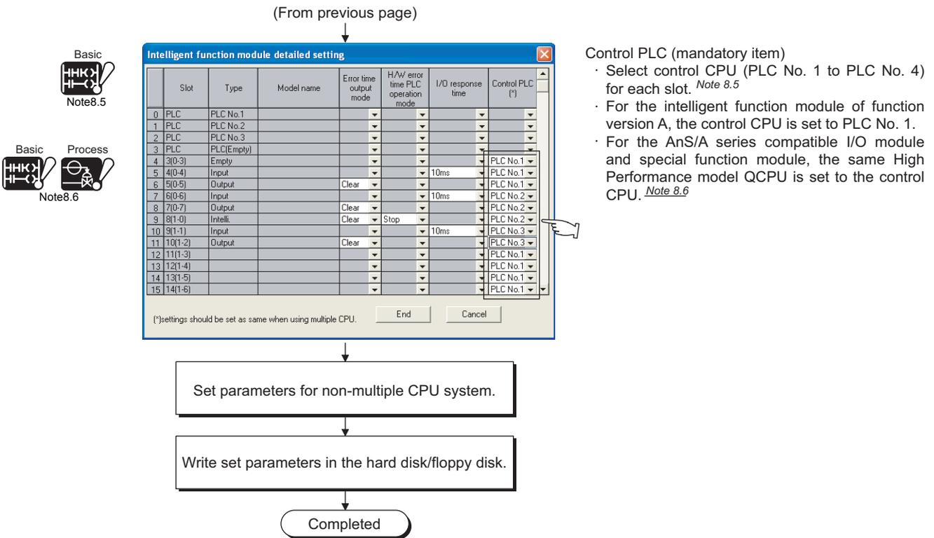
Diagram 8.4 Parameter setting procedure for new multiple CPU system creation
