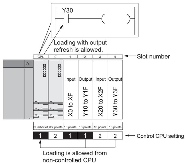
Diagram 3.21 When performing output loading in CPU No.1
