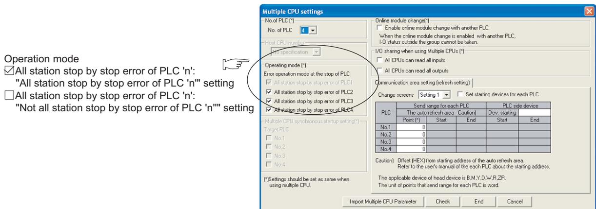
Diagram 3.31 Operation setting for stop error
