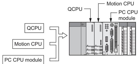
**Diagram 1.1 Configuration of multiple CPU**
