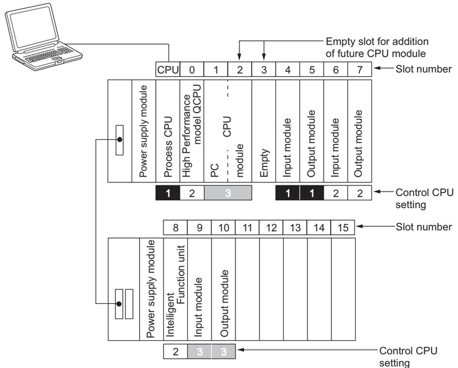
Diagram 8.2 Configuration example of multiple CPU system
