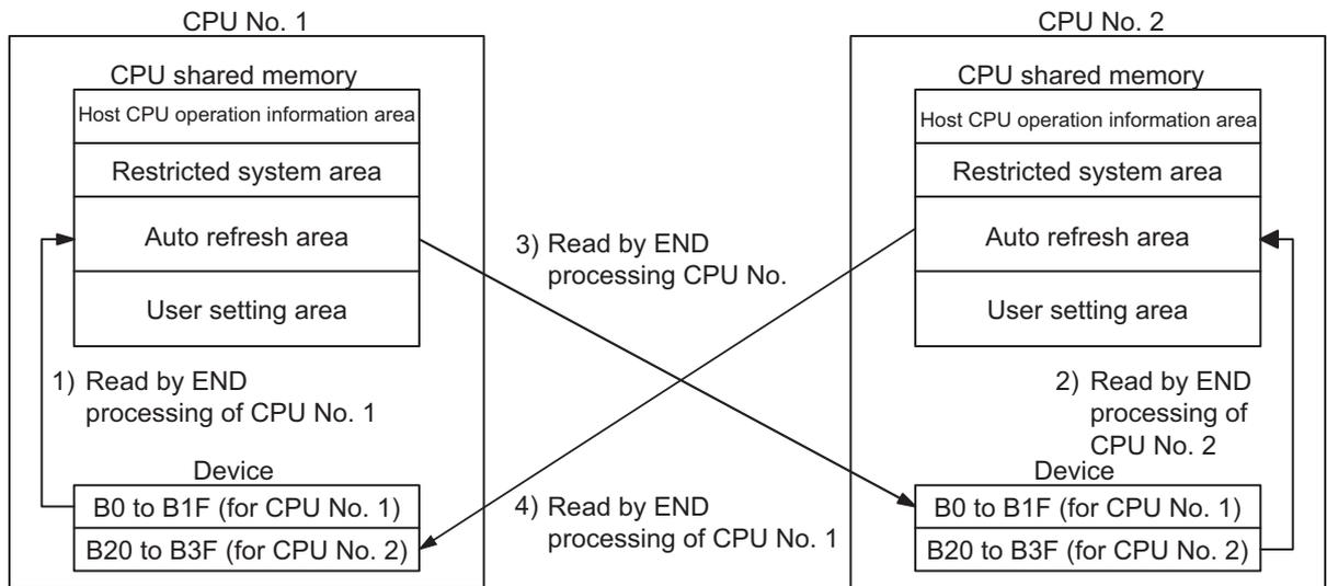
The processes performed during CPU No.1 END process.
