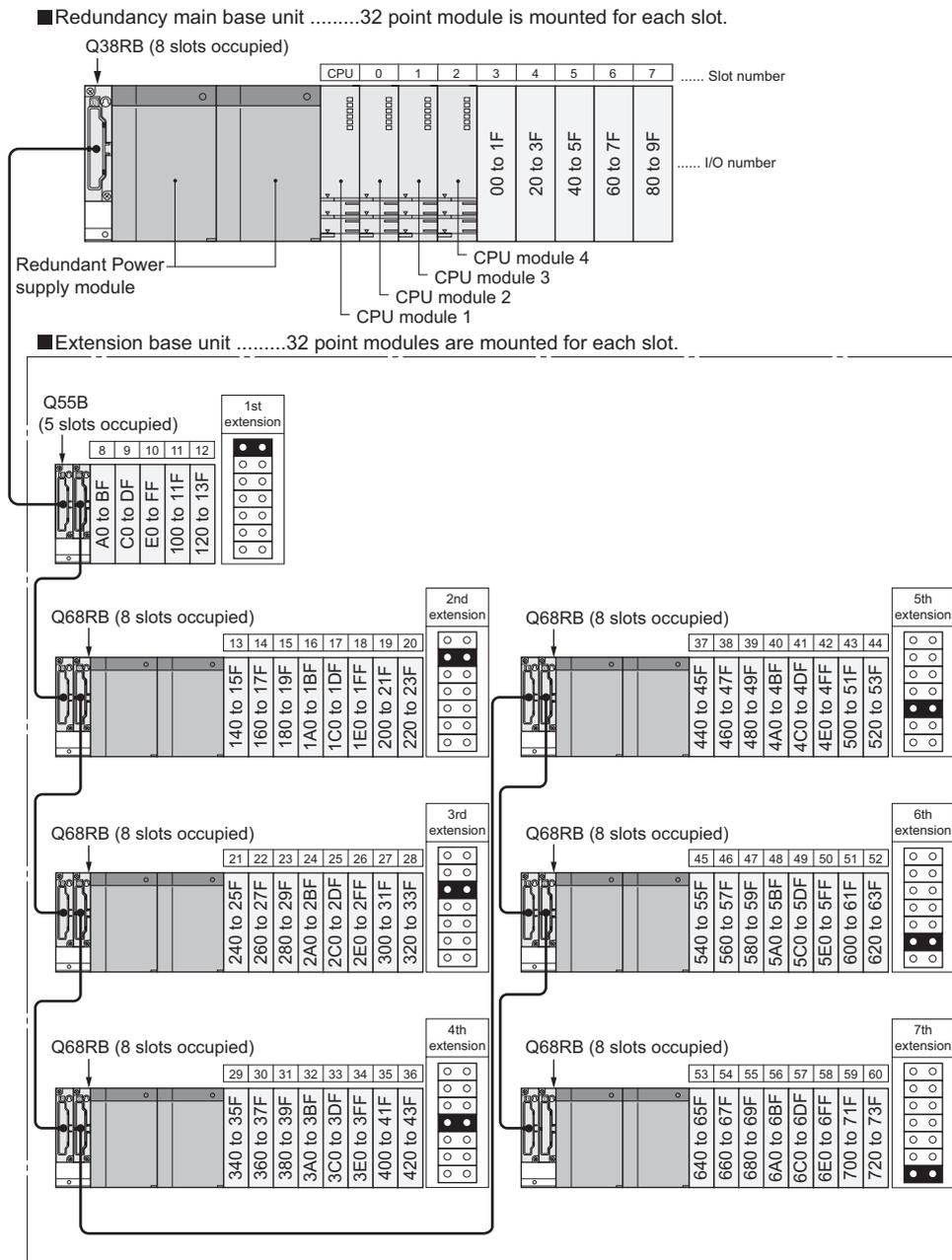
Diagram 2.18 System configuration example for using Q3□RB
