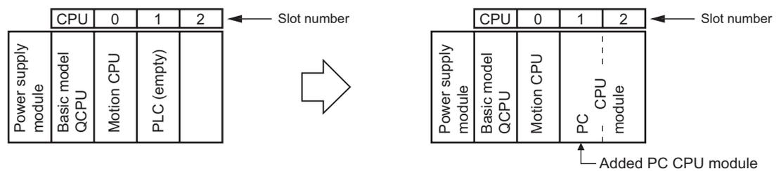
Diagram 3.3 "PLC (Empty)" setting for addition of PC CPU
