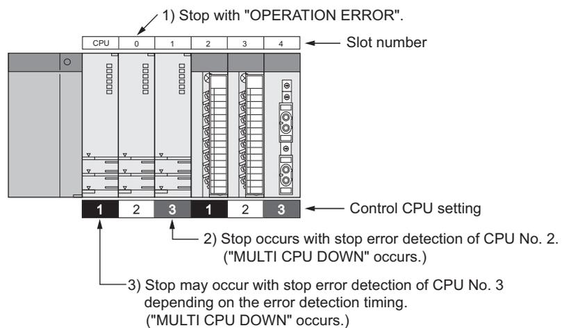
Diagram 3.32 Detection of stop error
