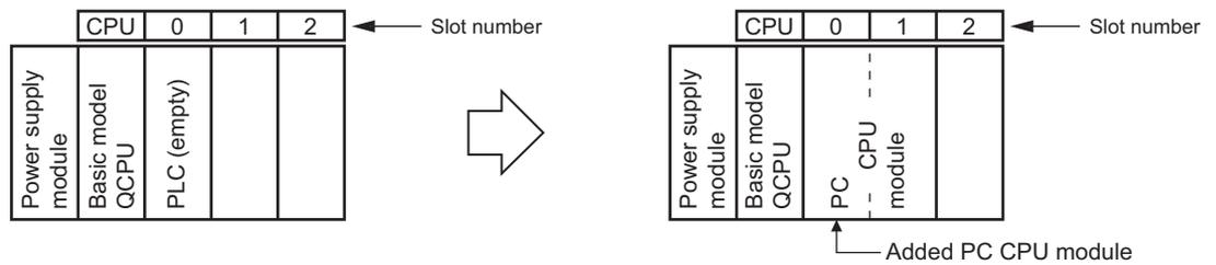
Diagram 3.4 "PLC (Empty)" setting for addition of PC CPU
