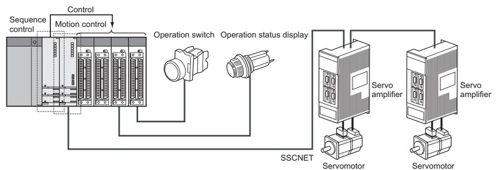
Diagram 1.4 Motion system configuration
