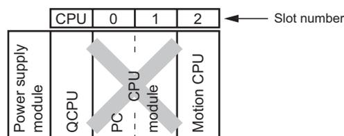
Diagram 3.10 Position where PC CPU module cannot be mounted
