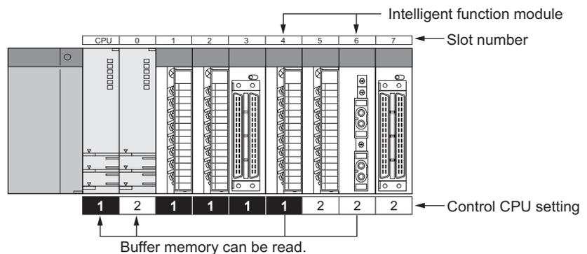
Diagram 3.23 Reading from intelligent function module
