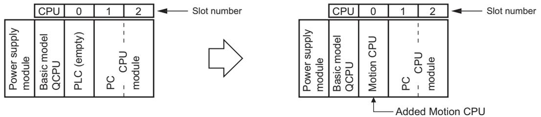
Diagram 3.5 "PLC (Empty)" setting between CPU modules
