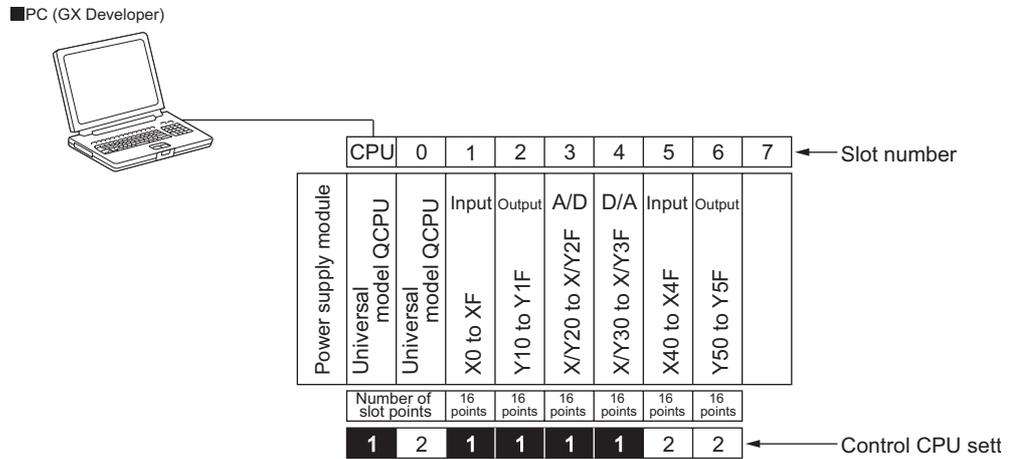
Diagram 8.18 Configuration example of multiple CPU system
