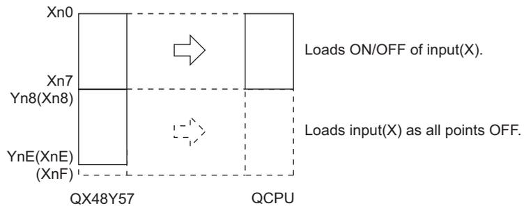
Diagram 3.19 Loading of input(X) from QX48Y57
