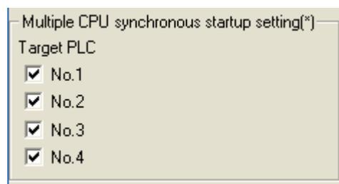
Diagram 4.25 Multiple CPU synchronized boot-up setting
