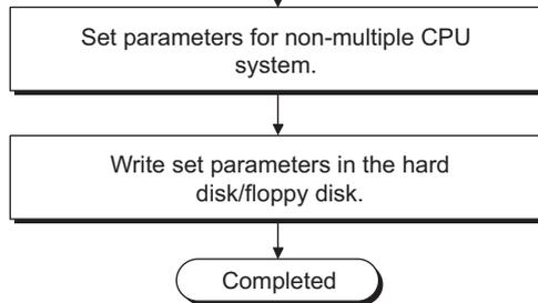
Diagram 8.9 Parameter setting procedure for reusing multiple CPU system parameters
