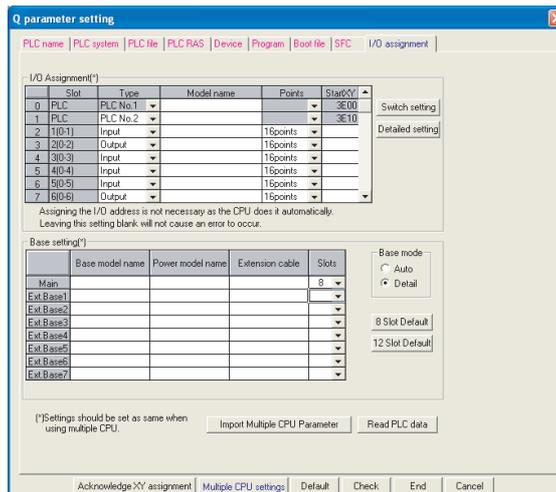
Diagram 8.11 I/O assignment settings of each module
