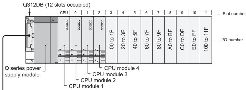
■ Extension base unit .....32 point modules are mounted for each slot.
