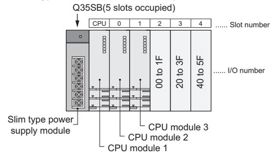
Diagram 2.20 System configuration example for using Q3□SB
