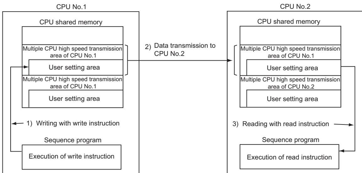
Procedure for the CPU No.2 to read device data of the CPU No.1
