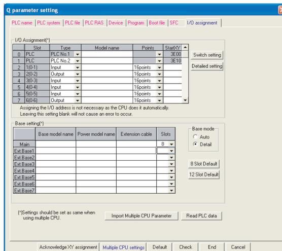
Diagram 8.19 I/O assignment settings of each module
