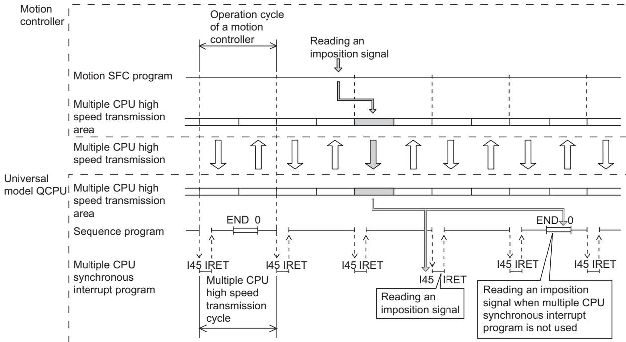
**Diagram 1.6 Reading data using multiple CPU synchronous interrupt program**
