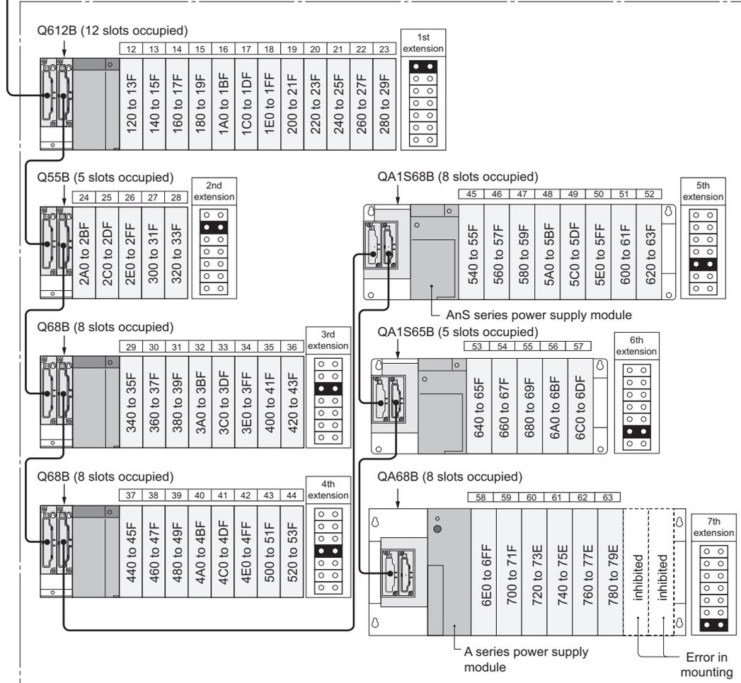
Diagram 2.6 System configuration example for using Q3□B
