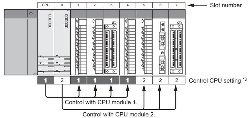
**Diagram 1.2 Setting of control CPU**
