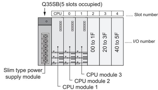
Diagram 2.10 System configuration example for using Q3□SB
