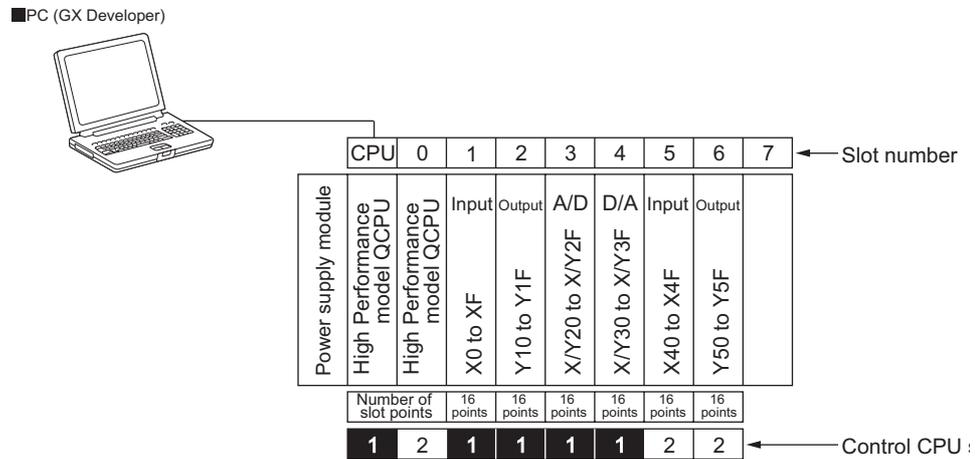
Diagram 8.10 Configuration example of multiple CPU system
