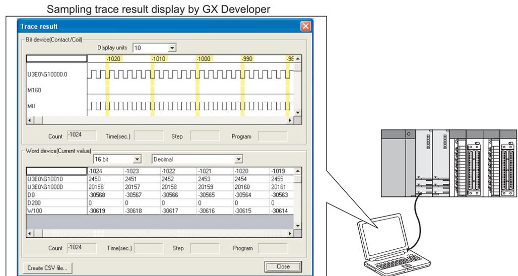
Diagram 1.7 Sampling trace at the time of configuring multiple CPU system
