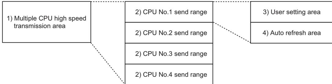
Diagram 4.5 Memory configuration of multiple CPU high speed transmission area
