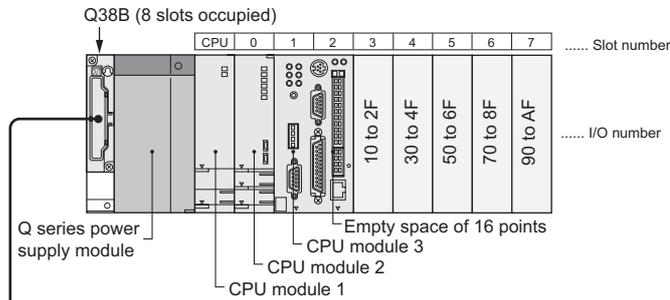
■ Extension base unit .....32 point modules are mounted for each slot.
