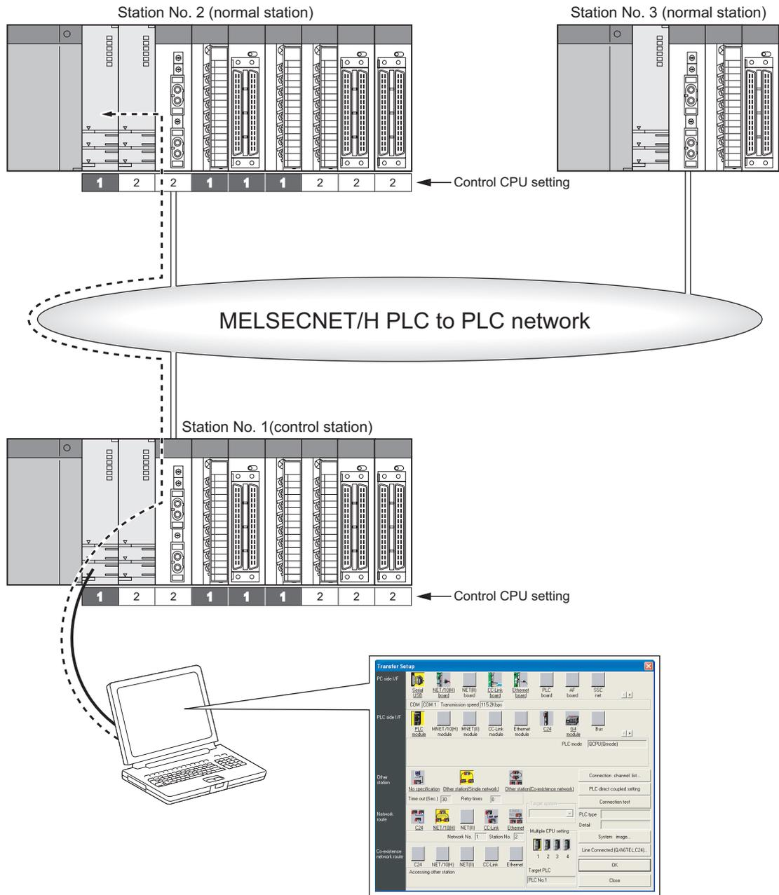
Diagram 3.29 Access through MELSECNET/H PLC to PLC network
