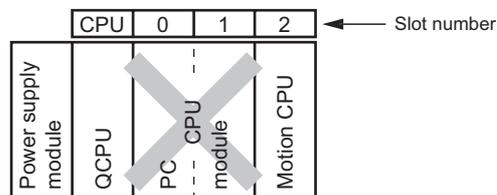
Diagram 3.7 Position where PC CPU module cannot be mounted
