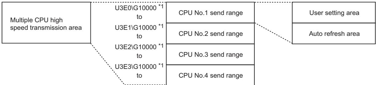
\* 1:Indicates addresses when user setting area for each CPU is specified using multiple CPU devices.
