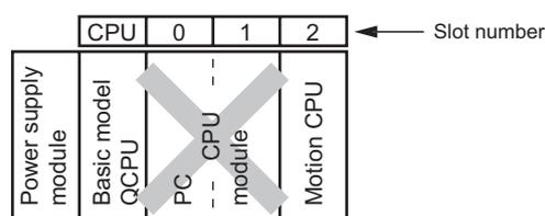
Diagram 3.1 Position where PC CPU module cannot be mounted
