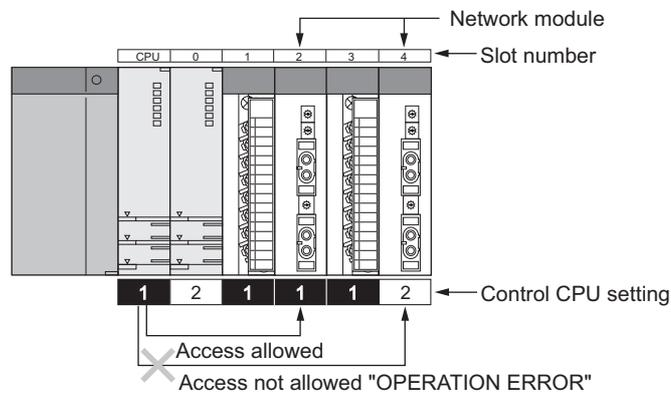
**Diagram 3.25 Access with instruction using link direct device**
