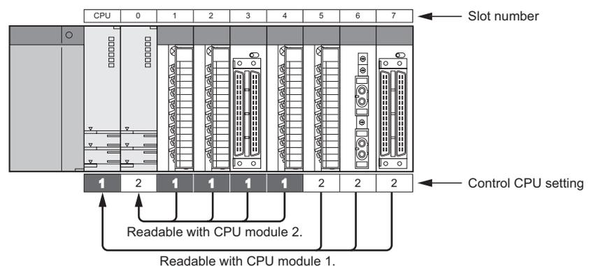
**Diagram 1.3 Access to non-controlled module**
