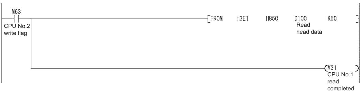
Diagram 8.17 Program example for continuously writing/reading data using the user setting area from CPU No. 2 to CPU No. 1
