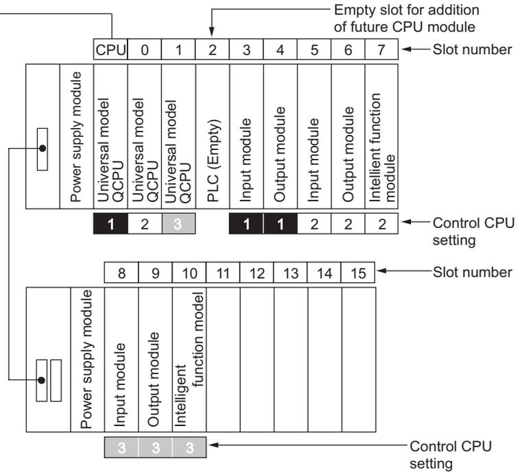
Diagram 8.6 Configuration example of multiple CPU system
