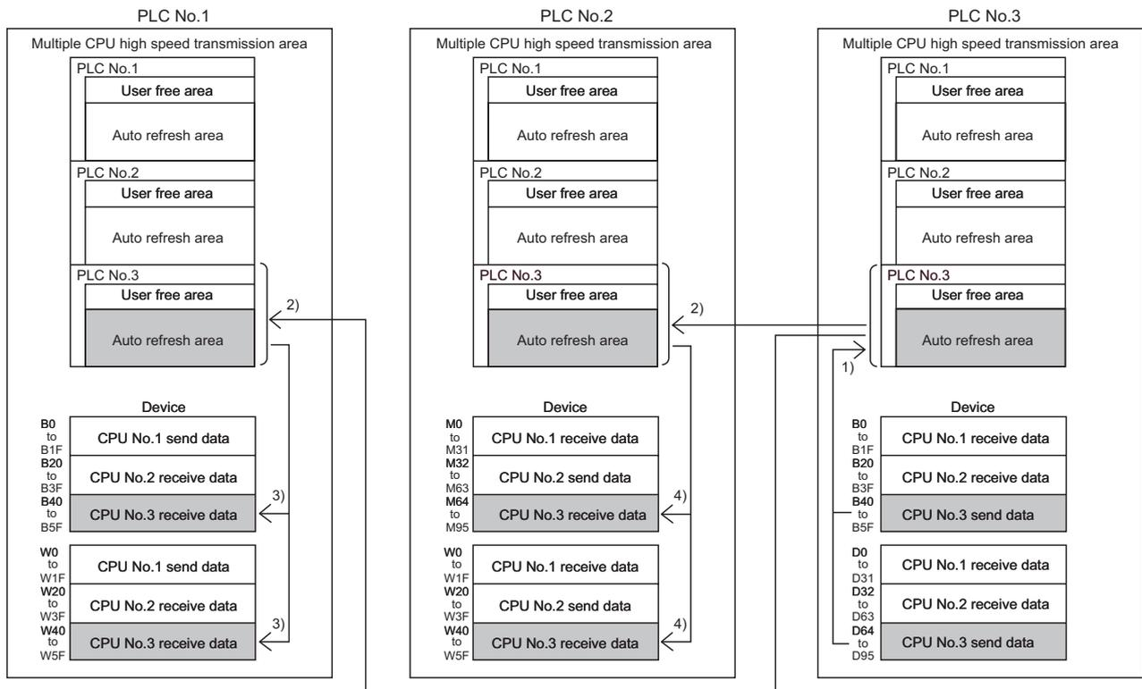
Diagram 4.33 Flow of sending data from CPU No.3 to other CPUs
