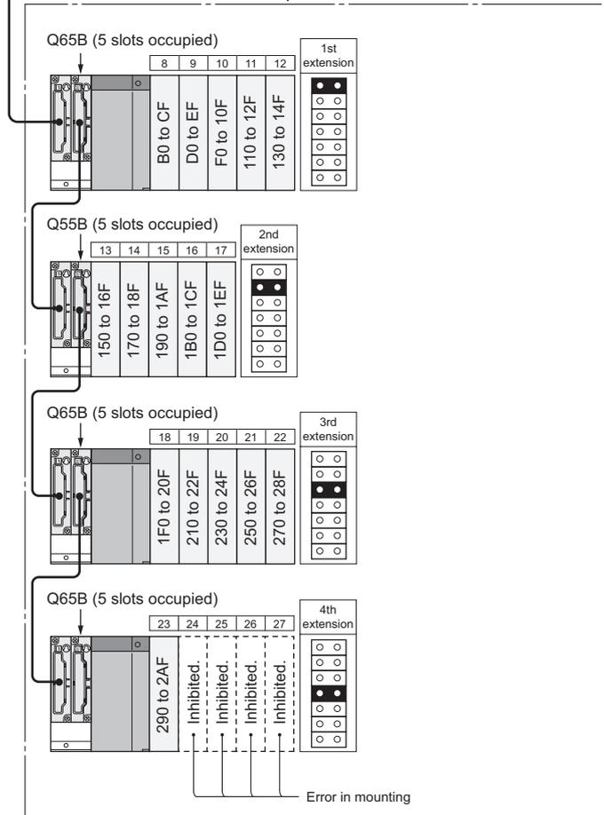
Diagram 2.2 System configuration example for using Basic model QCPU
