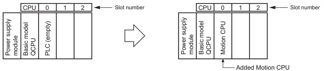
Diagram 3.2 "PLC (Empty)" setting for addition of Motion CPU
