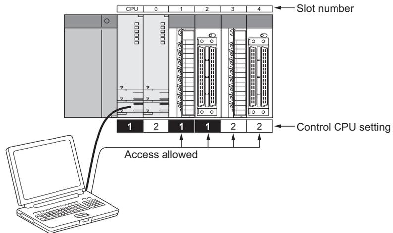
Diagram 3.28 Access to controlled module and non-controlled module
