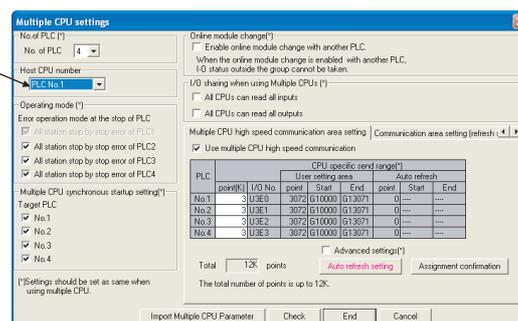
Diagram 3.34 Example of setting host CPU number of multiple CPU system
