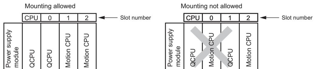
Diagram 3.6 Mounting position of Motion CPU
