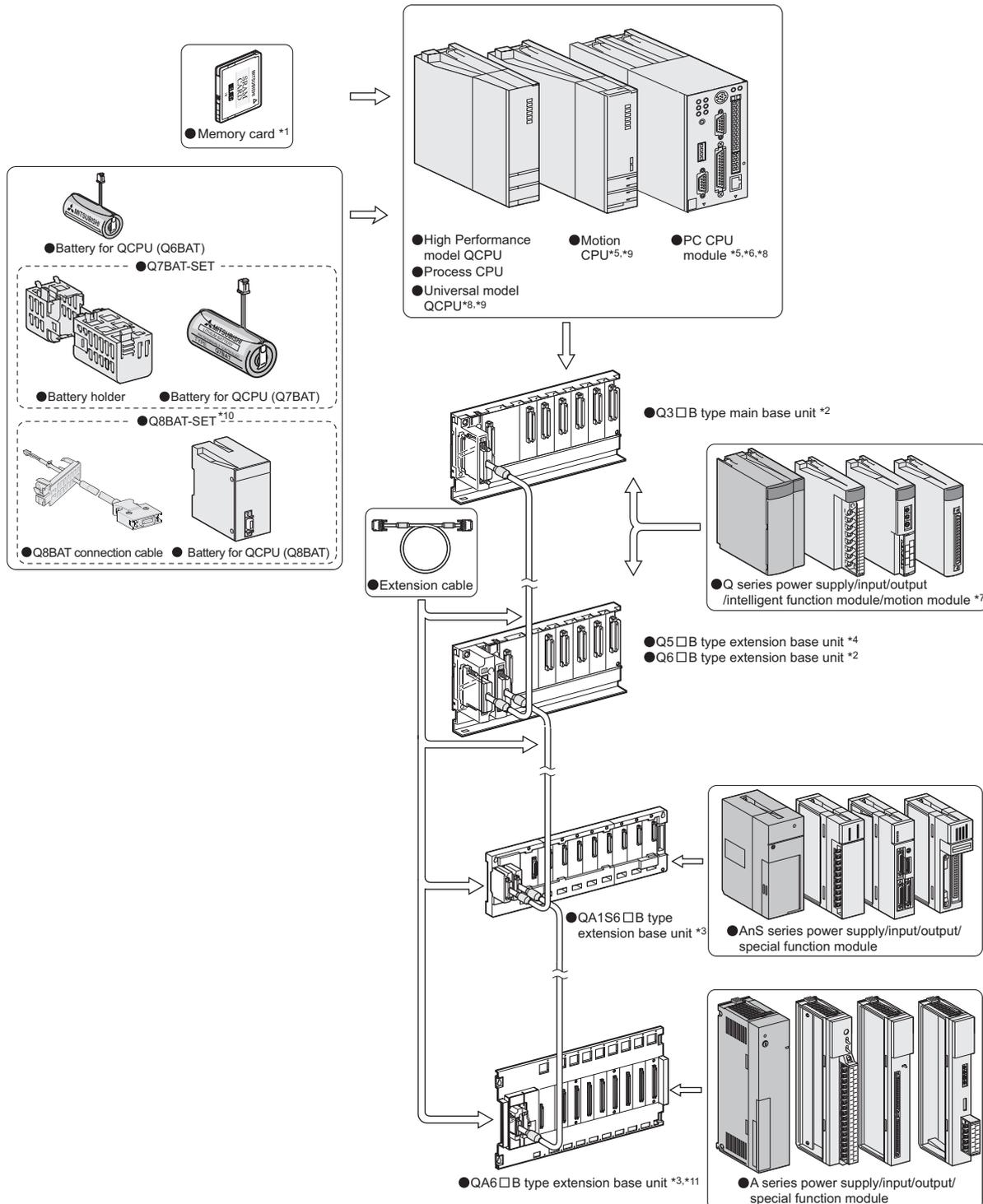
Diagram 2.5 System configuration when Q3□B is used
