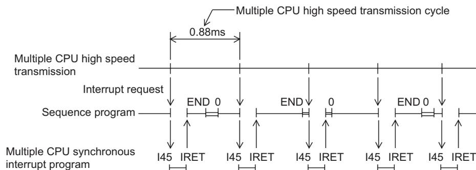
Diagram 4.46 Execution timing of multiple CPU synchronous interrupt program
