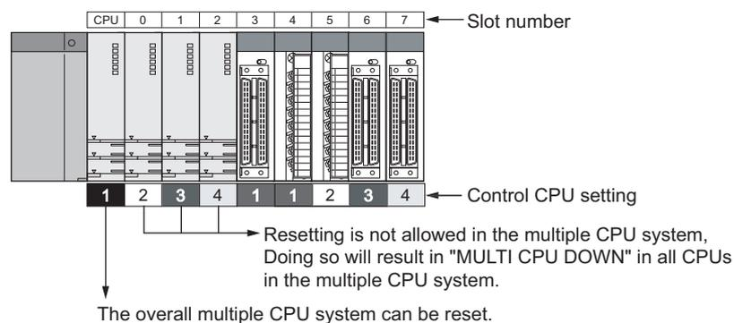
Diagram 3.30 Resetting of multiple CPU system
