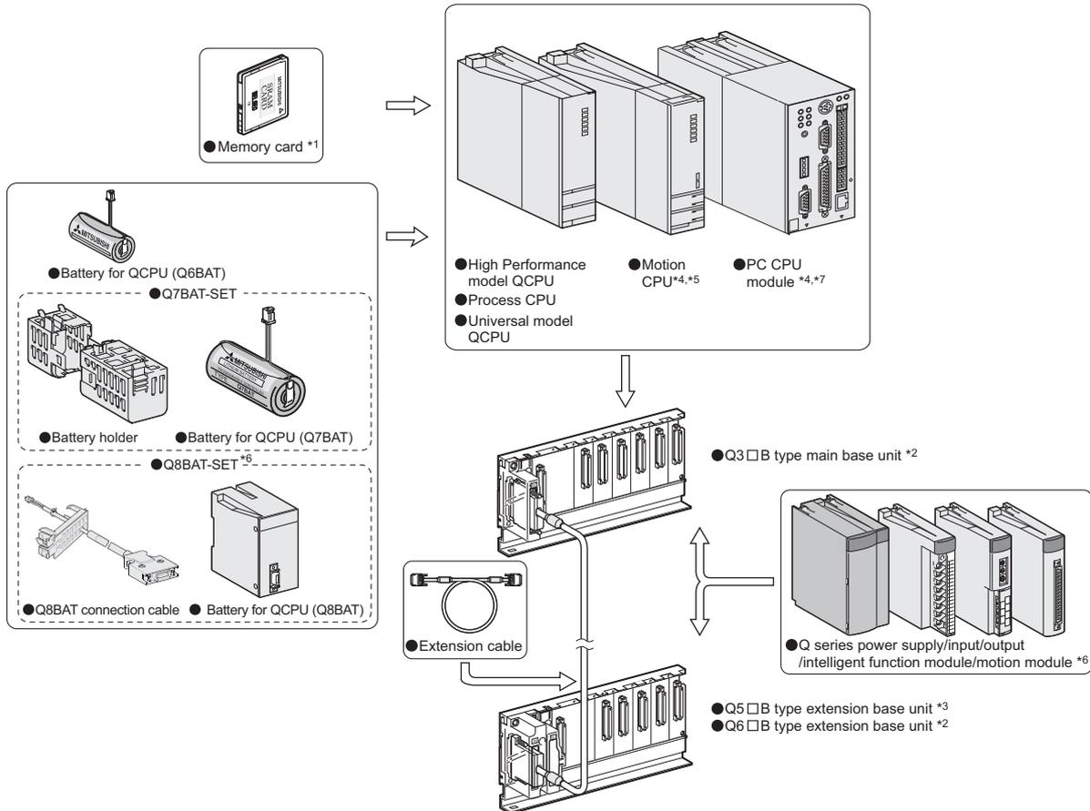
Diagram 2.15 System configuration when Q3□B is used
