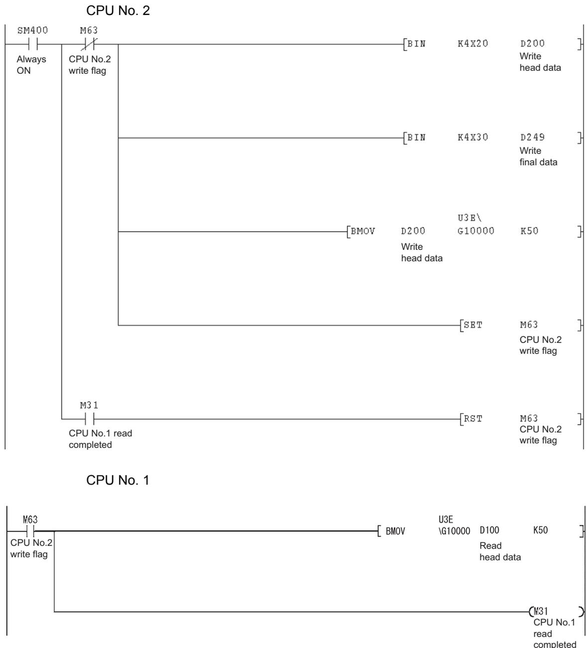
Diagram 8.24 Program example for continuously writing/reading data using the user setting area from CPU No. 2 to CPU No. 1
