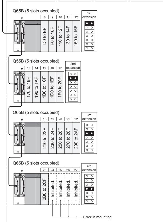
Diagram 2.4 System configuration example for using Basic model QCPU
