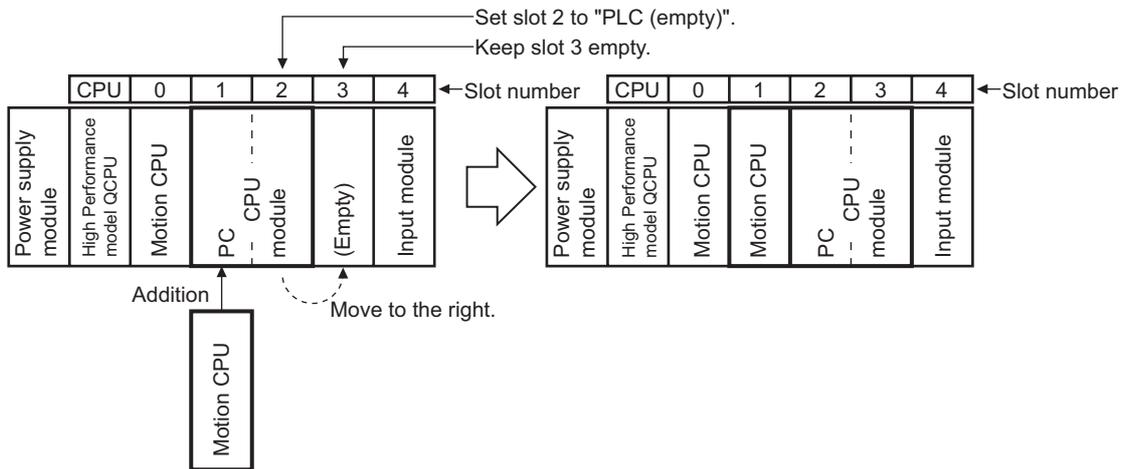
Diagram 3.9 Addition of Motion CPU when PC CPU module is mounted
