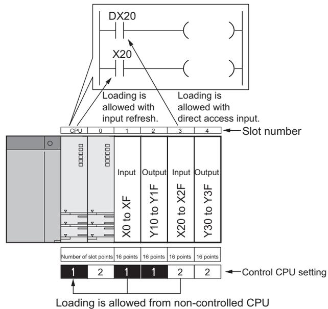
Diagram 3.18 When performing input loading in CPU No.1
