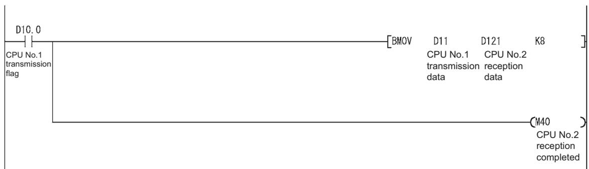
Diagram 8.14 Program example for storing data continuously from CPU No. 1 to CPU No. 2
