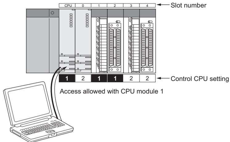
Diagram 3.26 Access to QCPU (when target CPU is not specified)
