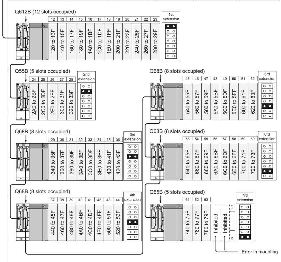
Diagram 2.12 System configuration example for using Q3□DB
