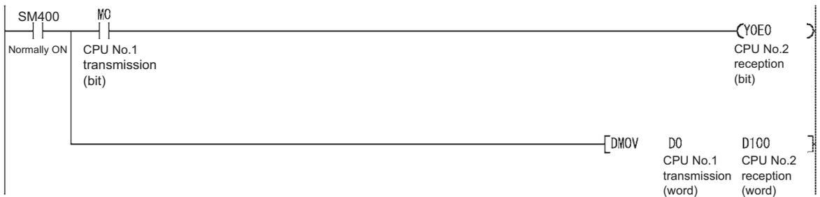
Diagram 8.21 Program example for sending bit and word data from CPU No. 1 to CPU No. 2
