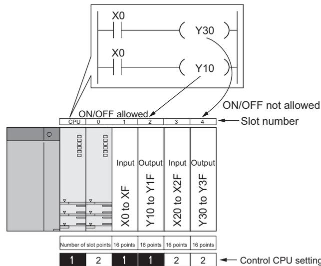
Diagram 3.22 When performing output from CPU No.1 to module
