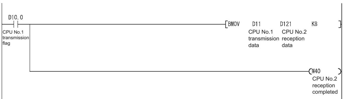
Diagram 8.22 Program example for storing data continuously from CPU No. 1 to CPU No. 2
