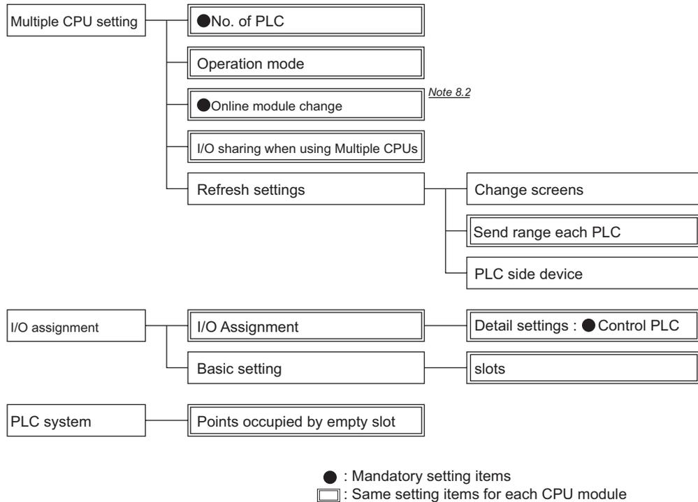
**Diagram 8.3 List of parameters required for multiple CPU system**
