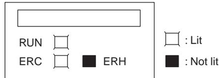
The ERC and RUN indicators will be lit when an error occurs while the Unit is operating normally. The following alarm flags will turn ON in CIO word n+9. These alarm flags will turn OFF automatically when the error is cleared.
