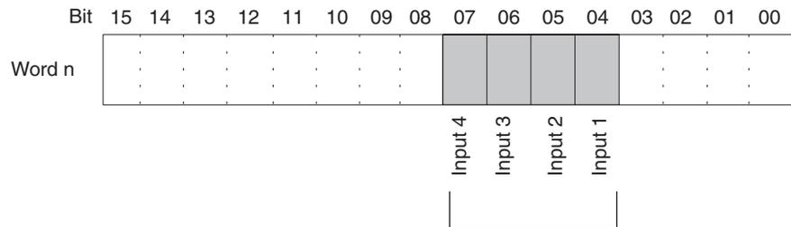
The peak value hold function will be in effect for the above input numbers while their respective bits are ON. The conversion values will be reset when the bits are turned OFF.
