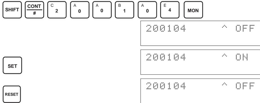
While the Offset Bit is ON, the offset value will be saved to the Unit's EEPROM when the Set Bit turns ON.
