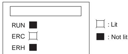
The ERC indicator will be lit when the initial settings for the Analog I/O Unit are not set correctly. The alarm flags for the following errors will turn ON in
