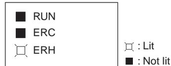
The unit number for the Analog Output Unit has not been set correctly.
