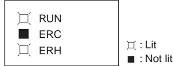
The ERH and RUN indicators will be lit if an error occurs in the I/O bus causing a WDT (watchdog timer) error in the CPU Unit, resulting in incorrect I/O refresh with the Analog Output Unit.
