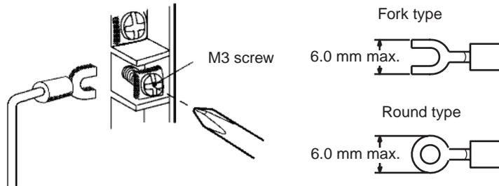
Connecting shielded cable to the Unit's AG terminals (A8, B8) can improve noise resistance.
