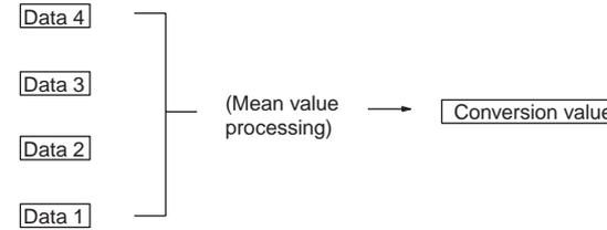
$$\text{Mean value} = (\text{Data 4} + \text{Data 3} + \text{Data 2} + \text{Data 1}) \div 4$$
