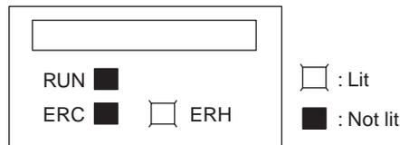
The unit number for the Analog Output Unit has not been set correctly.
