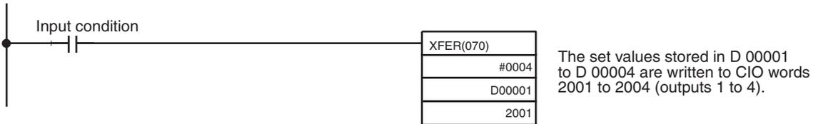
**Note** If the set value has been written outside the specified range, an output setting error will occur, and the value set by the output hold function will be output.
