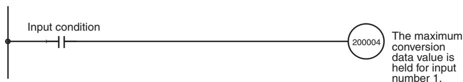
When mean value processing is used together with the peak value hold function, the mean value will be held.
