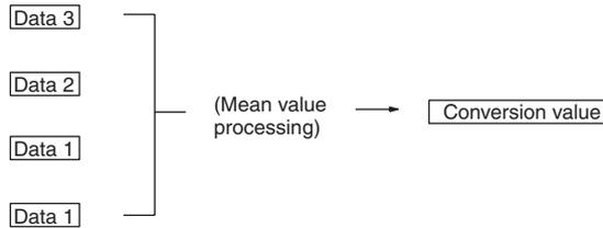
$$\text{Mean value} = (\text{Data 3} + \text{Data 2} + \text{Data 1} + \text{Data 1}) \div 4$$
