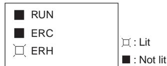
The unit number for the Analog Input Unit has not been set correctly.
