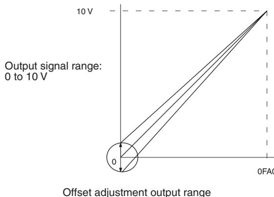
The following example uses output number 1 adjustment for illustration. (The unit number is 0.)
