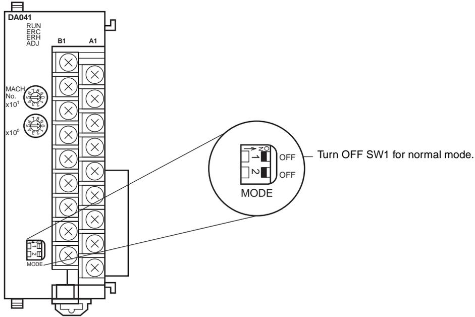
2. Set the unit number switch. Refer to 5-3-2 *Unit Number Switch* for further details.
