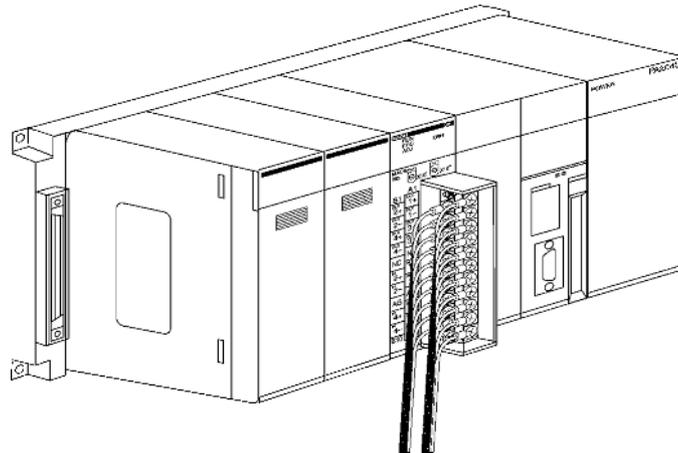
4. Set the unit number switch. Refer to 6-3-2 Unit Number Switch for further details.
