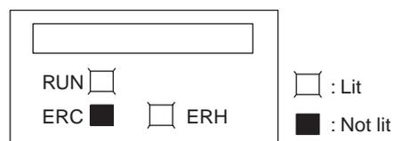
The ERH and RUN indicators will be lit if an error occurs in the I/O bus causing a WDT (watchdog timer) error in the CPU Unit, resulting in incorrect I/O refresh with the Analog Output Unit.
