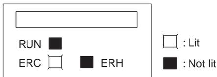
The ERC indicator will be lit when the initial settings for the Analog I/O Unit are not set correctly. The alarm flags for the following errors will turn ON in CIO word n+9. These alarm flags will turn OFF when the error is cleared and
