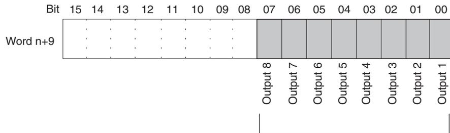
When a setting error is detected for a particular output, the corresponding bit turns ON. When the error is cleared, the bit turns OFF.
