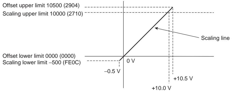
The following table shows the correspondence between input signals and converted scaling values. (The values shown in parentheses are binary data.)
