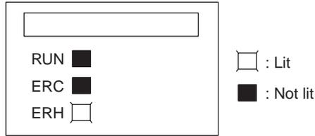
The unit number for the Analog I/O Unit has not been set correctly.
