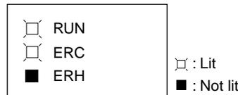
The ERC and RUN indicators will be lit when an error occurs while the Unit is operating normally. The following alarm flags will turn ON in CIO word n+9. These alarm flags will turn OFF automatically when the error is cleared.
