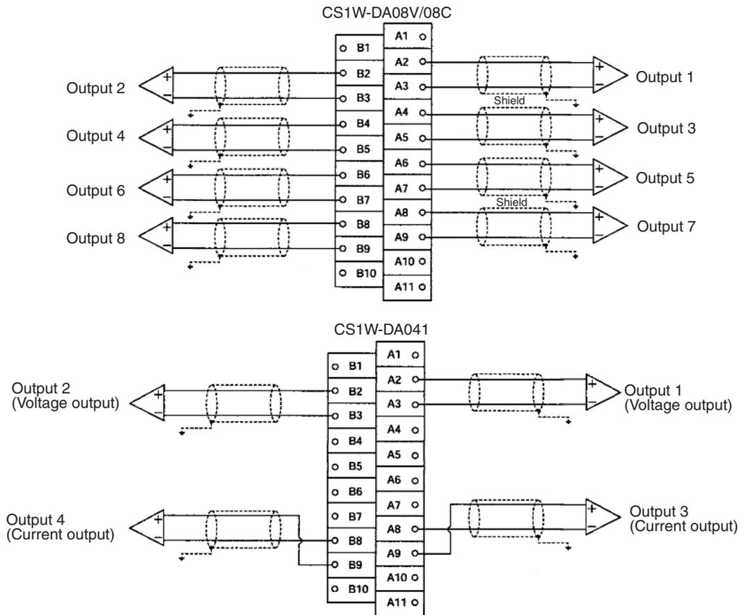
**Note** Crimp-type terminals must be used for terminal connections, and the screws must be tightened securely. Use M3 screws and tighten them to a torque of 0.5 N·m.
