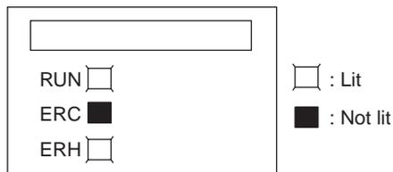
The ERH and RUN indicators will be lit if an error occurs in the I/O bus causing a WDT (watchdog timer) error in the CPU Unit, resulting in incorrect I/O refresh with the Analog I/O Unit.
