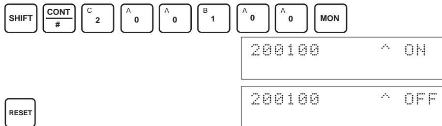
**Caution** Do not turn OFF the power supply or restart the Unit while the Set Bit is ON (data is being written to the EEPROM). Otherwise, illegal data may be written in the Unit's EEPROM and "EEPROM Errors" may occur when the power supply is turned ON or when the Unit is restarted, causing a malfunction.
