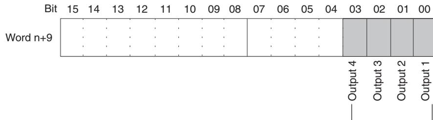
When a setting error is detected for a particular output, the corresponding bit turns ON. When the error is cleared, the bit turns OFF.
