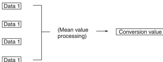
$$\text{Mean value} = (\text{Data 1} + \text{Data 1} + \text{Data 1} + \text{Data 1}) \div 4$$
