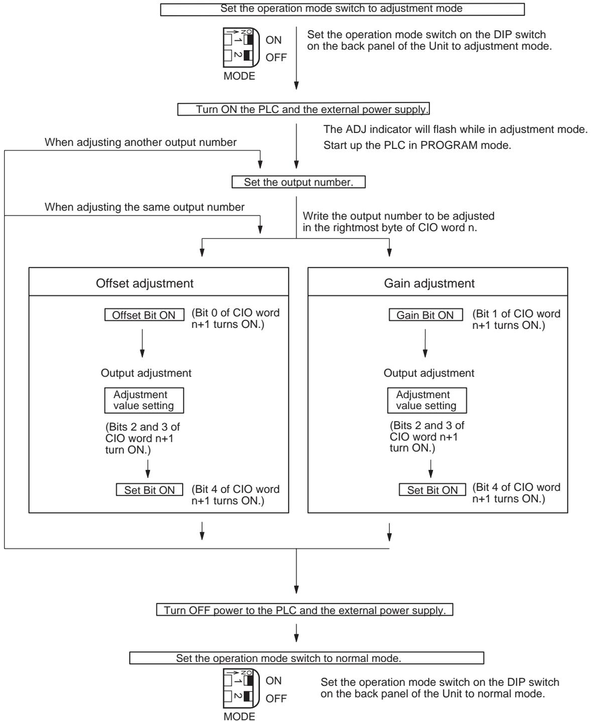
**Caution** Be sure to turn OFF the power to the PLC before changing the setting of the operation mode switch.
