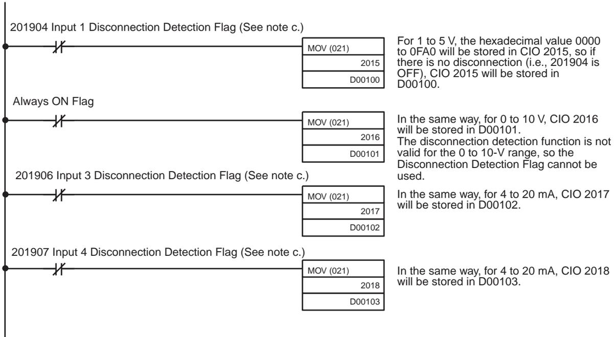
c) The input Disconnection Detection Flag is allocated to bits 04 to 07 of word (n + 9). Refer to *Allocations for Normal Mode* on page 302 and *7-6-6 Input Disconnection Detection Function* for further details.
