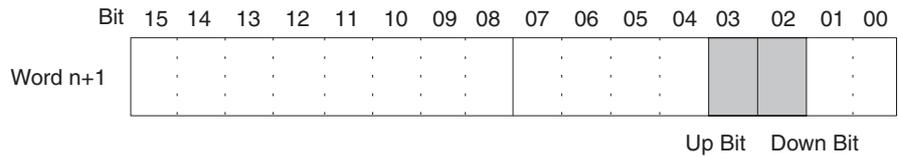
While the Up Bit is ON, the set value will be increased by 1 resolution every 0.5 seconds. After it has been ON for 3 seconds, the set value will be increased by 1 resolution every 0.1 seconds.
