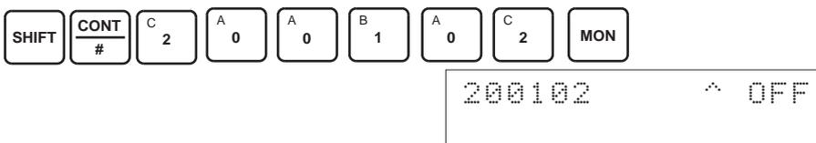
The bit will remain ON until the output voltage becomes an appropriate value, at which time, the output will turn OFF.
