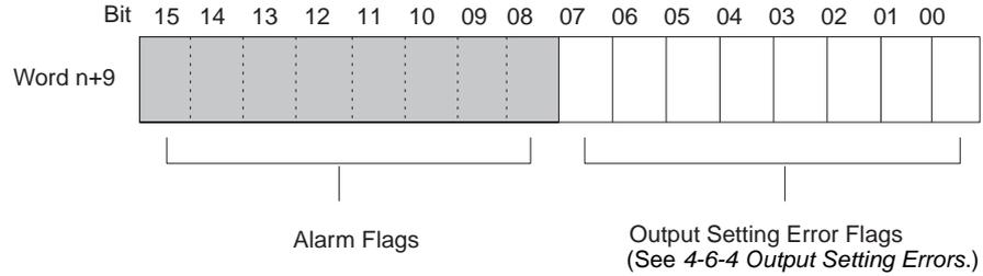
**Note** With the CS1W-DA041, the Output Setting Error Flags are bits 00 to 03.
