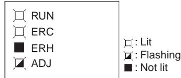
This alarm will occur in the case of incorrect operation while in the adjustment mode. In adjustment mode, the Adjustment Mode ON Flag will turn ON in bit 15 of CIO word n+9.
