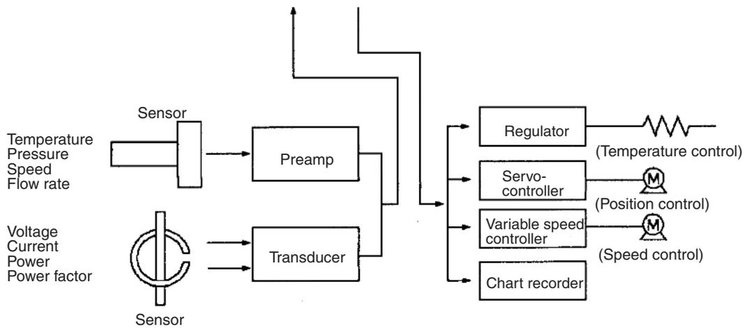
**Note** The above diagram is an installation example for the CS1W-AD081(-V1) Analog Input Unit and CS1W-DA08V Analog Output Unit.
