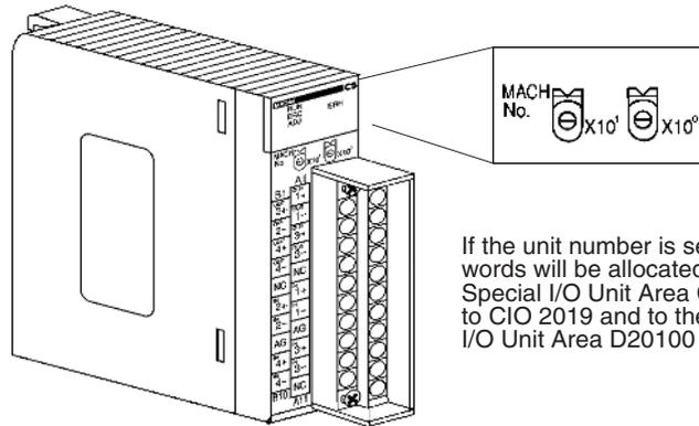
If the unit number is set to 1, words will be allocated to the Special I/O Unit Area CIO 2010 to CIO 2019 and to the Special I/O Unit Area D20100 to D20199.
