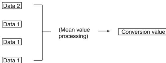
$$\text{Mean value} = (\text{Data 2} + \text{Data 1} + \text{Data 1} + \text{Data 1}) \div 4$$
