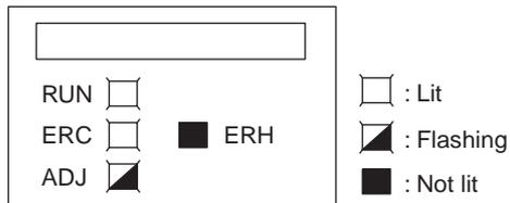
This alarm will occur in the case of incorrect operation while in the adjustment mode. In adjustment mode, the Adjustment Mode ON Flag will turn ON in bit 15 of CIO word n+9.
