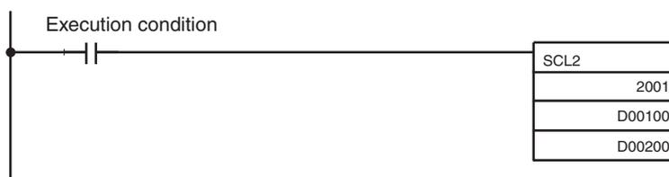
The value of word CIO 2005 is scaled according to the linear function calculated using the offset (0000 Hex), and the values of ΔX (1068 Hex) and ΔY (0315 Hex). The scaled value is then stored in word D00200.
