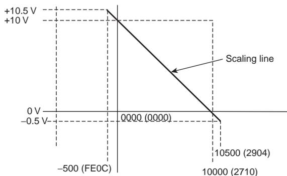
The following table shows the correspondence between output signals and converted scaling values. (The values shown in parentheses are 16-bit binary data.)
