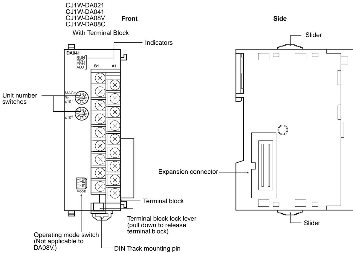
The terminal block is attached by a connector. It can be removed by pressing down on the lever at the bottom of the terminal block. Be sure that this lever is raised during normal operation.
