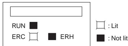
The ERC indicator will be lit when the initial settings for the Analog Output Unit are not set correctly. The alarm flags for the following errors will turn ON in CIO word n+9. These alarm flags will turn OFF when the error is cleared and the Unit is restarted, or the Special I/O Unit Restart Bit is turned ON and then OFF again.
