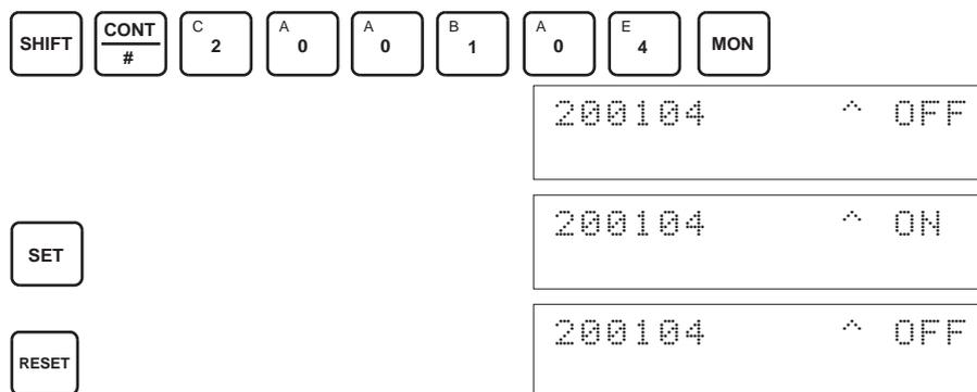
While the Offset Bit is ON, the offset value will be saved to the Unit's EEPROM when the Set Bit turns ON.
