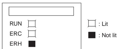
The ERC and RUN indicators will be lit when an error occurs while the Unit is operating normally. The following alarm flags will turn ON in CIO word n+9. These alarm flags will turn OFF automatically when the error is cleared.
