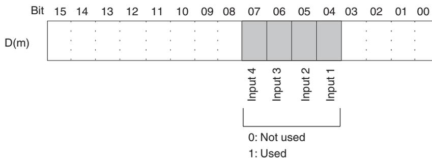
The analog input sampling interval can be shortened by setting any unused input numbers to 0.
