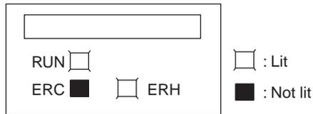
The ERH and RUN indicators will be lit if an error occurs in the I/O bus causing a WDT (watchdog timer) error in the CPU Unit, resulting in incorrect I/O refresh with the Analog I/O Unit.
