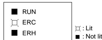
The ERC indicator will be lit when the initial settings for the Analog Output Unit are not set correctly. The alarm flags for the following errors will turn ON in CIO word n+9. These alarm flags will turn OFF when the error is cleared and the Unit is restarted, or the Special I/O Unit Restart Bit is turned ON and then OFF again.
