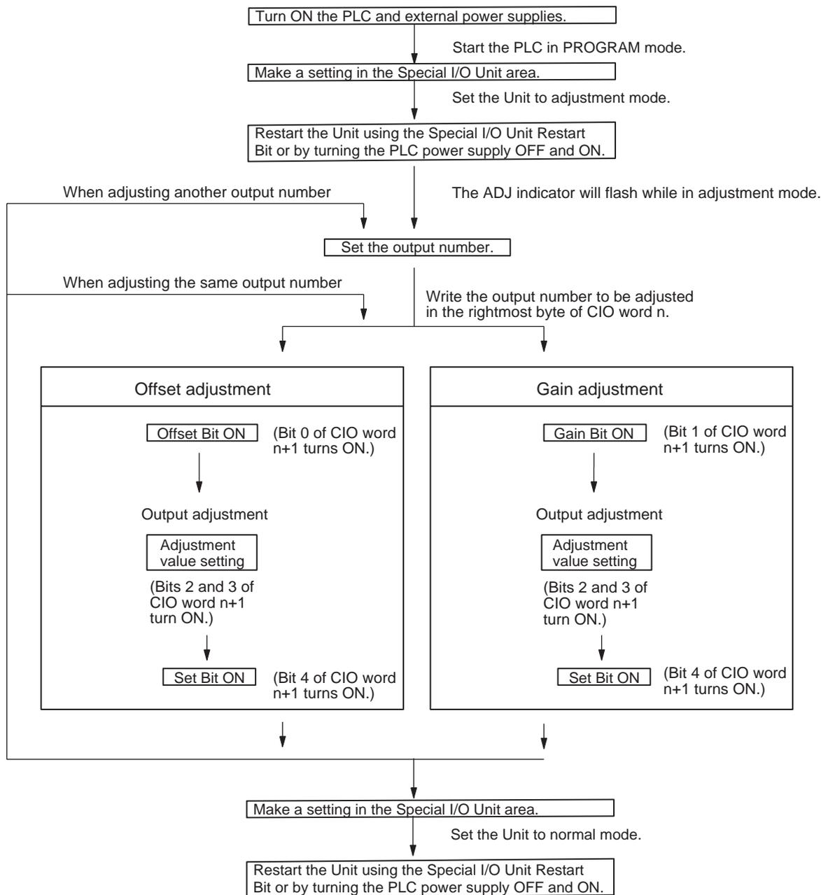
**⚠ Caution** Set the PLC to PROGRAM mode when using the Analog Output Unit in adjustment mode. If the PLC is in MONITOR mode or RUN mode, the Analog Output Unit will stop operating, and the output values that existed immediately before this stoppage will be retained.
