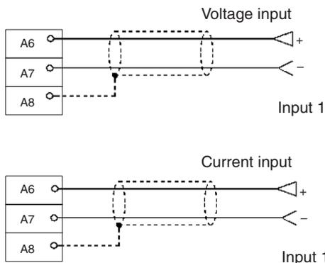
For current input, check that the voltage/ current switch is ON.
