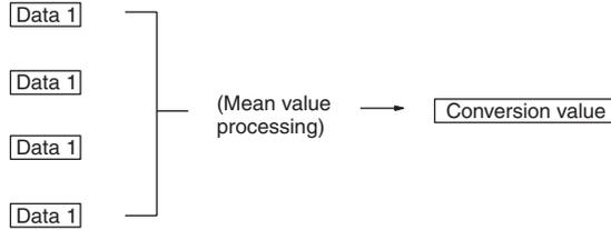
$$\text{Mean value} = (\text{Data 1} + \text{Data 1} + \text{Data 1} + \text{Data 1}) \div 4$$
