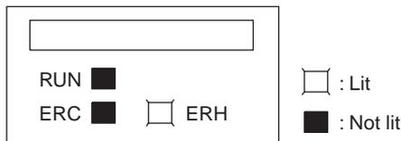
The unit number for the Analog I/O Unit has not been set correctly.
