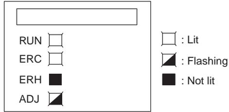
This alarm will occur in the case of incorrect operation while in the adjustment mode. In adjustment mode, the Adjustment Mode ON Flag will turn ON in bit 15 of CIO word n+9.
