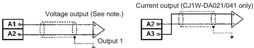
**Note** The output is current output when using a CJ1W-DA08C.
