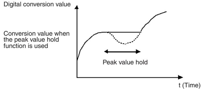
The peak value hold function can be set individually for each input number by turning on the respective bits (04 to 07) in CIO word n.
