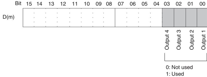
The analog output conversion cycle can be shortened by setting any unused output numbers to 0.
