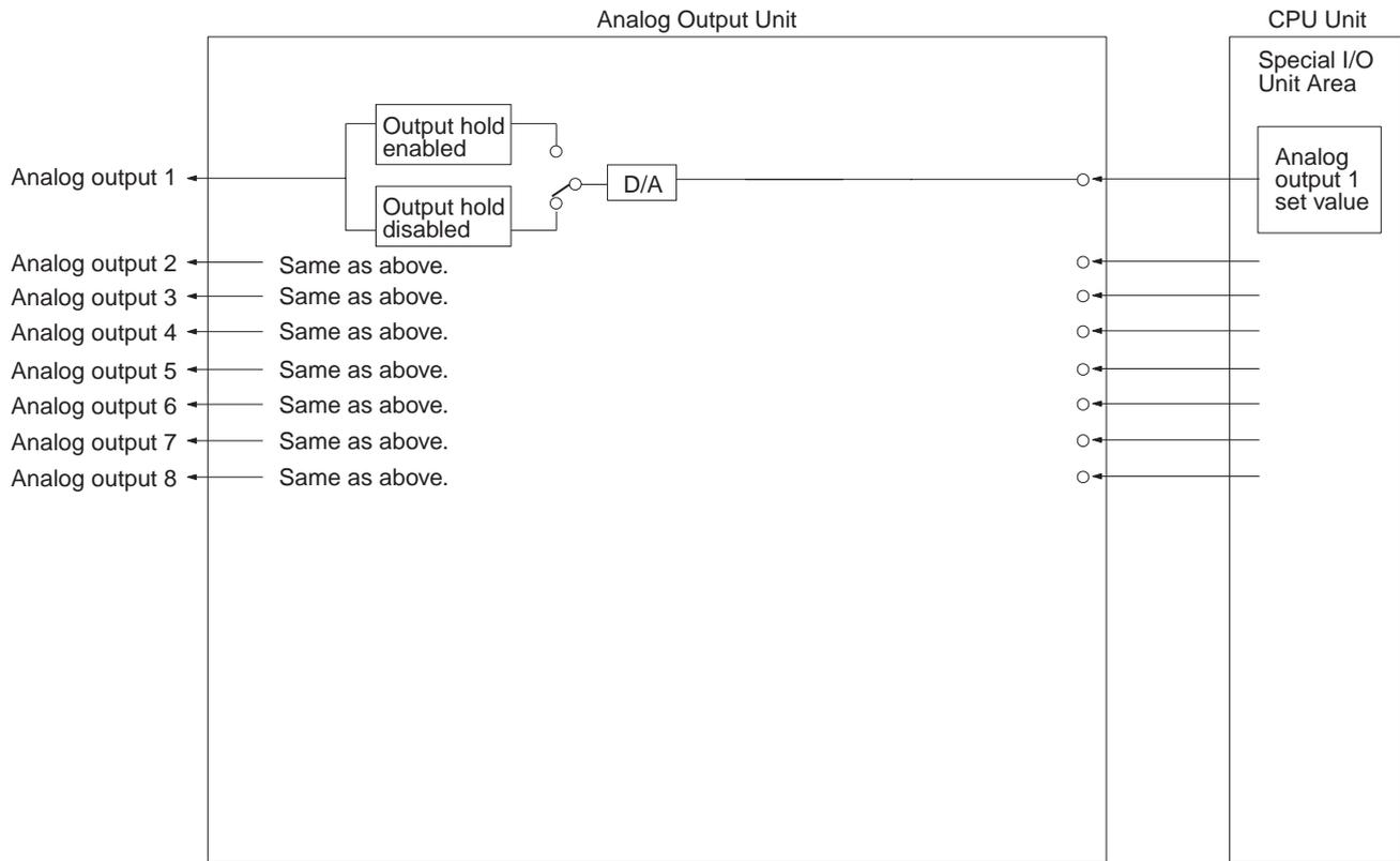
**Note** There are only four analog outputs for the CS1W-DA041.
