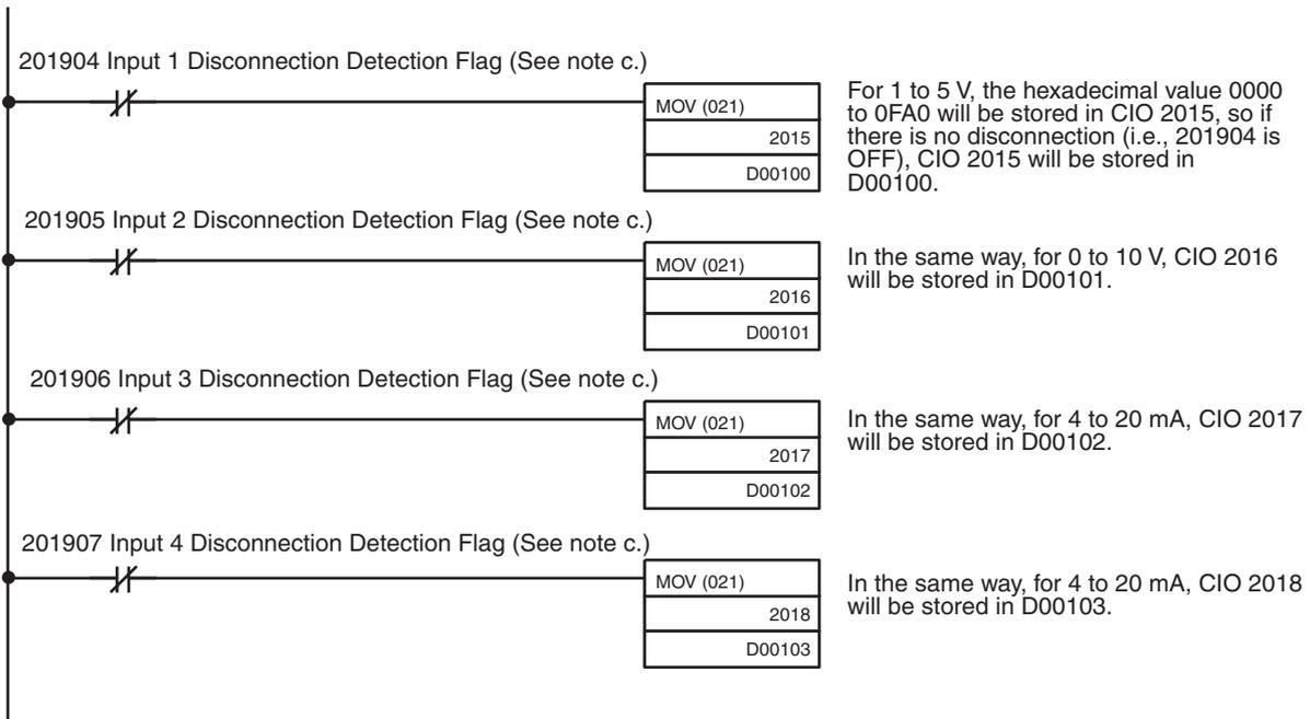
**c)** The input Disconnection Detection Flag is allocated to bits 04 to 07 of word (n + 9). Refer to *Allocations for Normal Mode* on page 236 and 6-6-4 *Input Disconnection Detection Function* for further details.
