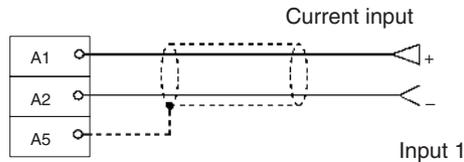
For current input, check that the voltage/current switch is ON.
