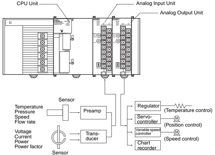
**Note** The above diagram is an installation example for the CJ1W-AD041-V1/081(-V1) Analog Input Unit and CJ1W-DA021/041 Analog Output Unit.
