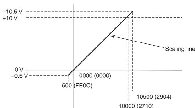
The following table shows the correspondence between output signals and converted scaling values. (The values shown in parentheses are 16-bit binary data.)
