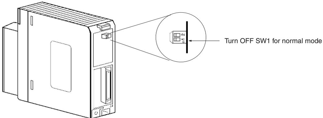
2. Mount and wire the Analog Output Unit. Refer to 1-2-1 Mounting Procedure, 4-4 Wiring or 4-4-3 Output Wiring Example for further details.
