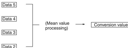
$$\text{Mean value} = (\text{Data 5} + \text{Data 4} + \text{Data 3} + \text{Data 2}) \div 4$$
