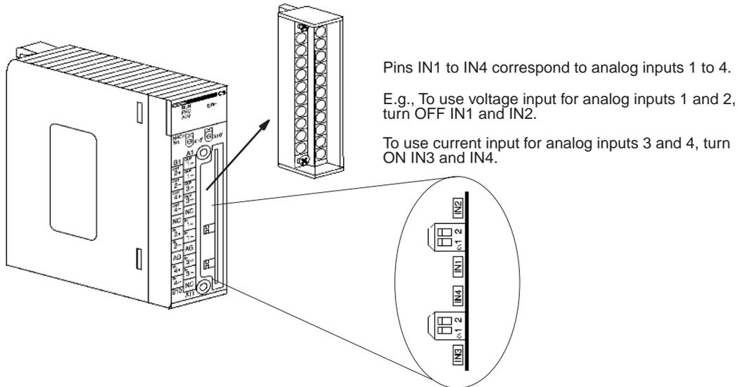
3. Mount and wire the Analog I/O Unit. Refer to 1-2-1 Mounting Procedure, 6-4 Wiring or 6-4-4 I/O Wiring Example for further details.
