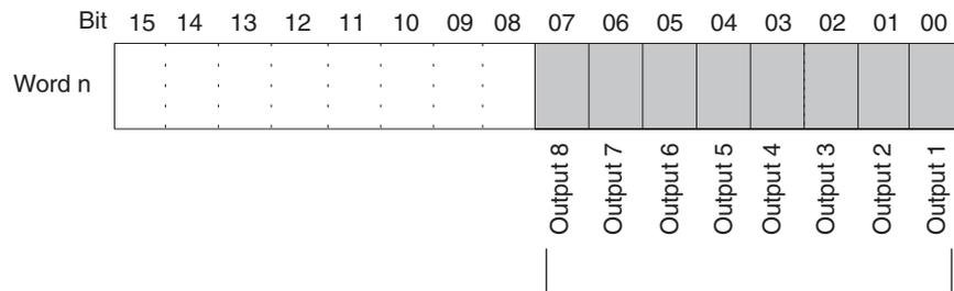
Analog conversion is executed while these bits are ON. When the bits are turned OFF, the conversion is stopped and the output data is held.
