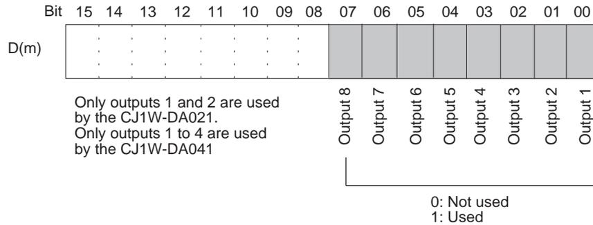
The analog output conversion cycle can be shortened by setting any unused output numbers to 0.
