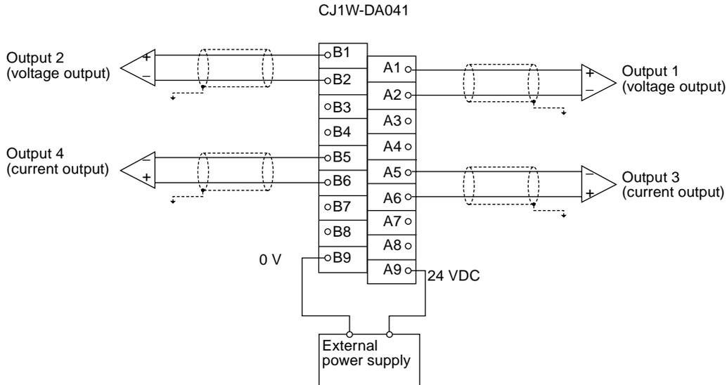
**Note** Crimp-type terminals must be used for terminal connections, and the screws must be tightened securely. Use M3 screws and tighten them to a torque of 0.5 N·m.
