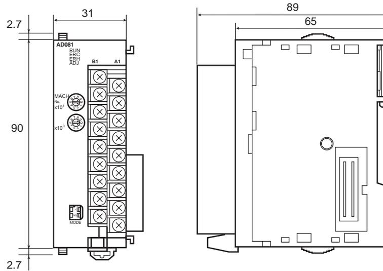
**CJ-series Unit Terminal Block Dimensions**
