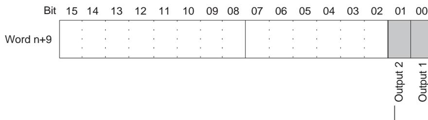
When a setting error is detected for a particular output, the corresponding bit turns ON. When the error is cleared, the bit turns OFF.
