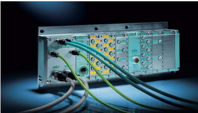
*SIMATIC ET 200pro with PROFINET connection and I/O modules*
