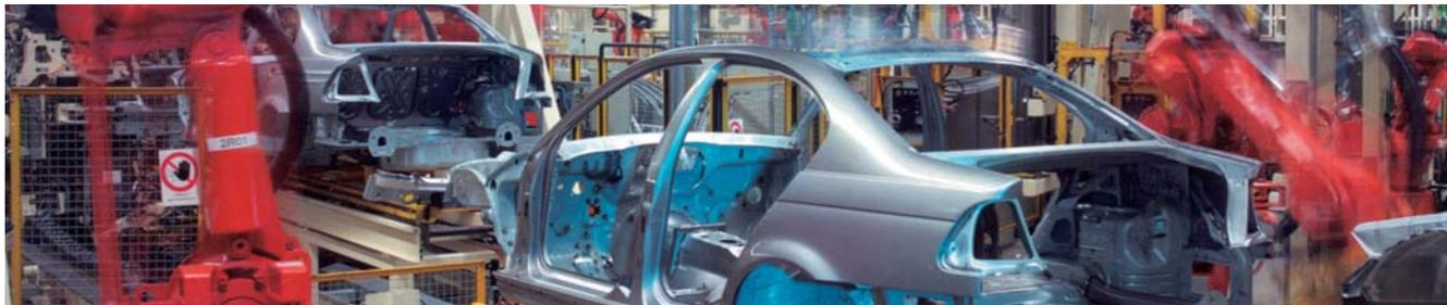
Production line in the automobile industry – automated with the SIMATIC S7-300
