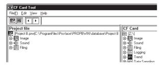
The image screen, sound data, Filing Data, Data-Transferring CSV file, startup system, backup data, dictionary file, and JPEG file will be copied from the CF Card to the designated Project's folder. Other data (alarm data, trend graph data, sampled data, logged data, etc.) must be copied using Windows Explorer or other similar software.
