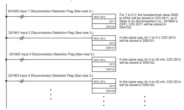
3. The input Disconnection Detection Flag is allocated to bits 00 to 07 of word (n + 9). Refer to *Allocations for Normal Mode* on page 88 for further details.
