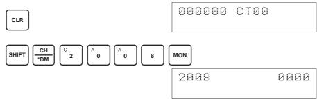
4. Change the set value so that the output voltage is as shown in the following table. The data can be set within the indicated ranges.
