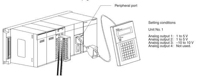
• The following diagram shows the output settings used. Refer to 4-6-1 Output Settings and Conversions for more details.
