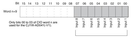
The respective bit turns ON when a disconnection is detected for a given input. When the disconnection is restored, the bit turns OFF.
