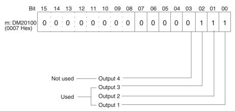
• The following diagram shows the output range settings. Refer to 4-6-1 Output Settings and Conversions for more details.
