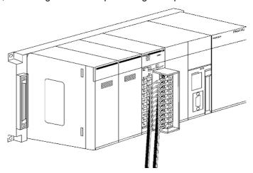
3. Set the unit number switch. Refer to *4-3-2 Unit Number Switch* for further details.
