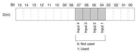
The analog input sampling interval can be shortened by setting any unused input numbers to 0.
