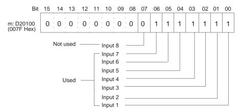
• The following diagram shows the input range settings. Refer to *DM Allocation Contents* on page 85 and 3-6-1 Input Settings and Conversion Values for more details.
