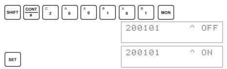
The analog input's digital conversion values while the Gain Bit is ON will be monitored in CIO word n+8.
