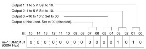
**Note** The output range setting is not required for the CJ1W-DA08C.
