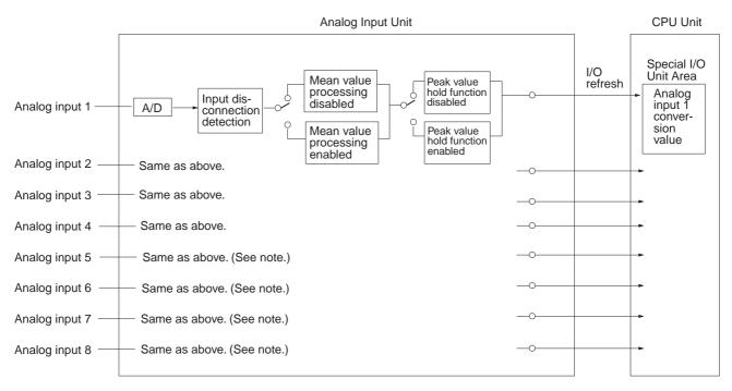
**Note** There are only four analog inputs for the CS1W-AD041(-V1).
