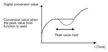
The peak value hold function can be set individually for each input number by turning on the respective bits (00 to 07 for CS1W-AD081(-V1), 00 to 03 for CS1W-AD041(-V1)) in CIO word n.
