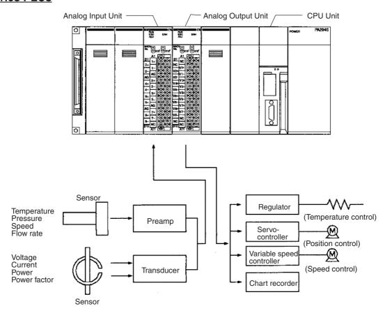
**Note** The above diagram is an installation example for the CS1W-AD081(-V1) Analog Input Unit and CS1W-DA08V Analog Output Unit.
