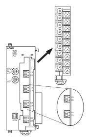
3. Set the unit number switch. Refer to 3-3-2 *Unit Number Switch* for further details.
