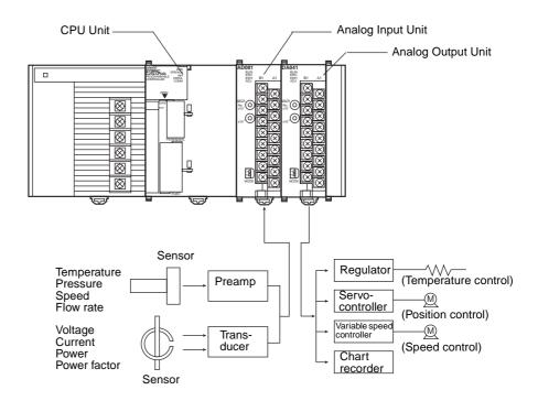
**Note** The above diagram is an installation example for the CJ1W-AD041-V1/081(-V1) Analog Input Unit and CJ1W-DA021/041 Analog Output Unit.
