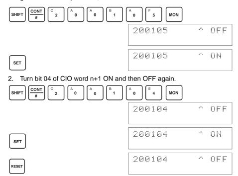
While the Clear Bit is ON, the adjusted value will be cleared and reset to the default offset and gain values when the Set Bit turns ON.
