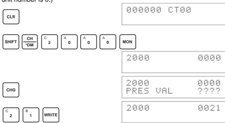
**Bits Used for Adjusting** Offset and Gain
