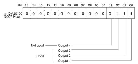
• The following diagram shows the output range settings. Refer to 5-6-1 Output Settings and Conversions for more details.
