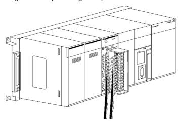
4. Set the unit number switch. Refer to 2-3-2 *Unit Number Switch* for further details.
