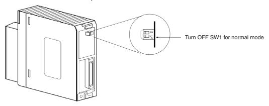
2. Mount and wire the Analog Output Unit. Refer to 1-2-1 Mounting Procedure, 4-4 Wiring or 4-4-3 Output Wiring Example for further details.
