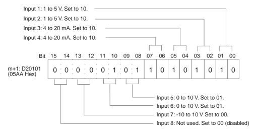
The following diagram shows the conversion time/resolution setting (version-1 Units only). (Refer to 2-6-2 Conversion Time/Resolution Setting.)
