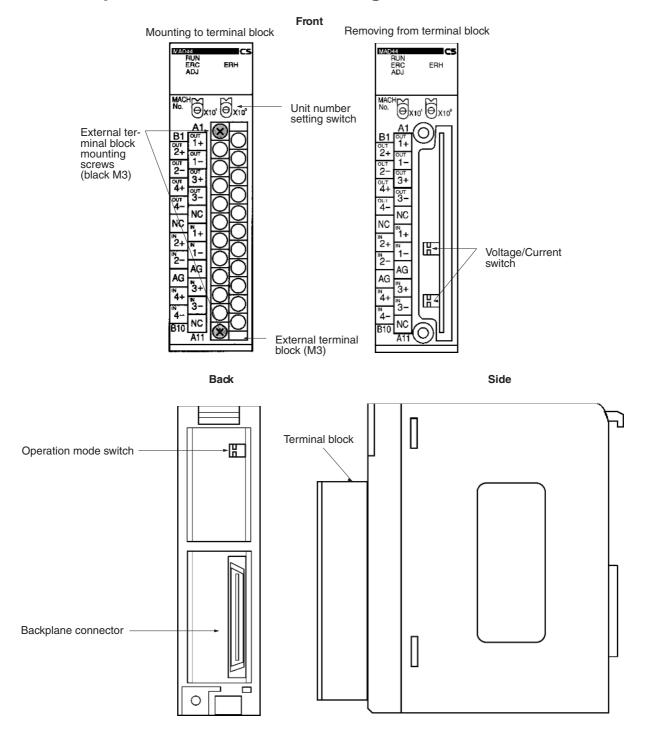
The terminal block is attached by a connector. It can be removed by loosening the two black mounting screws located at the top and bottom of the terminal block.
