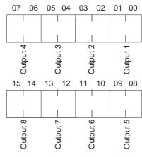
00: -10 to 10 V 01: 0 to 10 V 10: 1 to 5 V 11: 0 to 5 V
