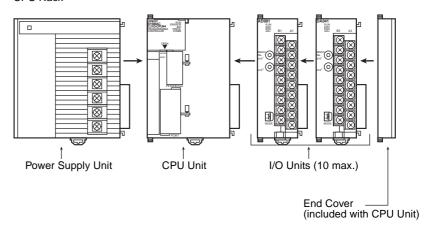
Use the following procedure to connect Analog I/O Units to a CJ-series Rack.
