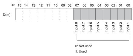
**Note** There are only four inputs for the CJ1W-AD041-V1.
