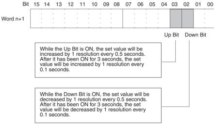
The following example increases the output voltage.
