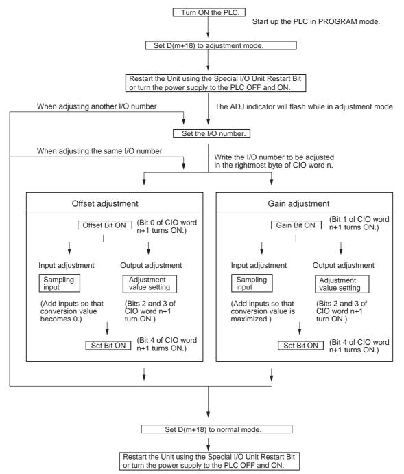
Caution Set the PLC to PROGRAM mode when using the Analog I/O Unit in adjustment mode. If the PLC is in MONITOR mode or RUN mode, the Analog I/O Unit will stop operating, and the input and output values that existed immediately before this stoppage will be retained.
