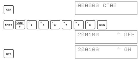
The analog input's digital conversion values while the Offset Bit is ON will be monitored in CIO word n+8.
