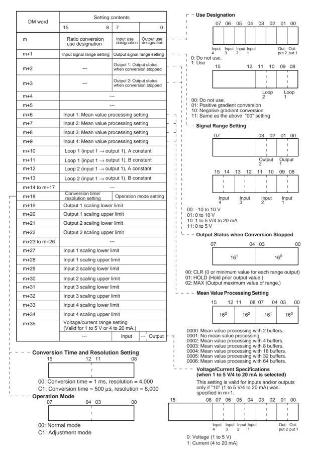
**Note** m=20000+ unit number x 100 is allocated as the DM number.
