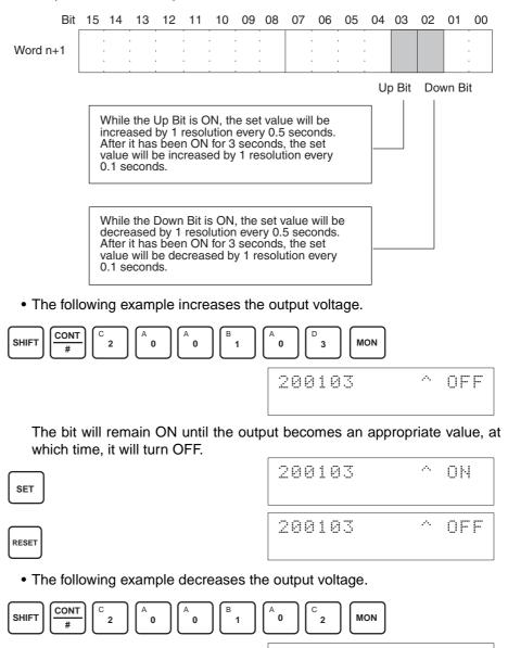
The bit will remain ON until the output becomes an appropriate value, at
