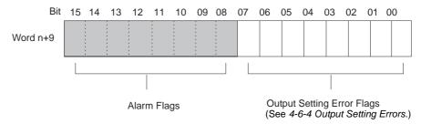
Note With the CS1W-DA041, the Output Setting Error Flags are bits 00 to 03.
