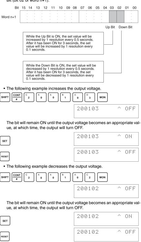
5. Check the 10V/5V output, and then turn bit 04 (the Set Bit) of CIO word n+1 ON and then OFF again.
