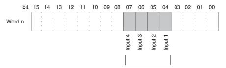
The peak value hold function will be in effect for the above input numbers while their respective bits are ON. The conversion values will be reset when the bits are turned OFF.
