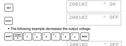
The bit will remain ON until the output becomes an appropriate value, at which time, it will turn OFF.
