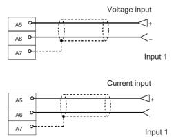
For current input, check that the voltage/current switch is ON.
