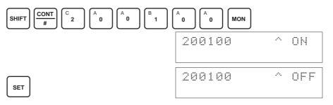
/!\ Caution Do not turn OFF the power supply or restart the Unit while the Set Bit is ON (data is being written to the EEPROM). Otherwise, illegal data may be written in the Unit's EEPROM and "EEPROM Errors" may occur when the power supply is turned ON or when the Unit is restarted, causing a malfunction.
