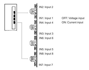
**Note** There are only four inputs for the CS1W-AD041(-V1).
