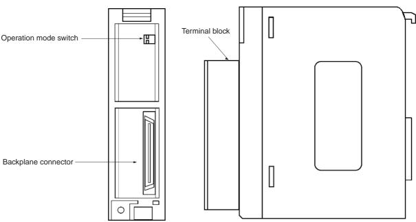
The terminal block is attached by a connector. It can be removed by loosening the two black mounting screws located at the top and bottom of the terminal block.
