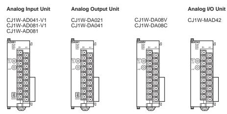
The CJ-series Analog I/O Units are Special I/O Units that enable highly accurate analog input and output at a resolution of 4,000. The CJ1W-AD041/081 Analog Input Units convert analog signals to digital data and transmits it to CJ-series PLCs, whereas the CJ1W-DA041 Analog Output Unit converts digital data from CJ-series PLCs to analog format for output.
