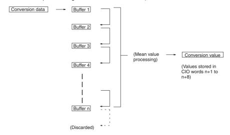
When "n" number of history buffers are being used, the first conversion data will be stored for all "n" number of history buffers immediately data conversion has begun or after a disconnection is restored.
