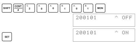
The analog input's digital conversion values while the Gain Bit is ON will be monitored in CIO word n+8.
