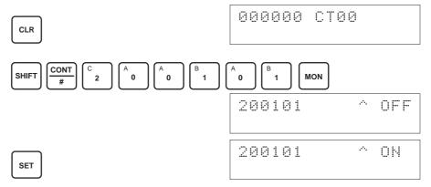
Check whether the output devices are connected.
