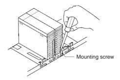
Leave enough space below each Rack, as shown in the following diagram for mounting and removing the Units.
