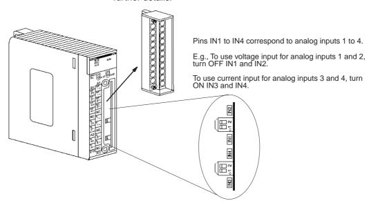
3. Mount and wire the Analog I/O Unit. Refer to 1-2-1 Mounting Procedure, 6-4 Wiring or 6-4-4 I/O Wiring Example for further details.
