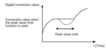
The peak value hold function can be set individually for each input number by turning on the respective bits (00 to 07) in CIO word n.
