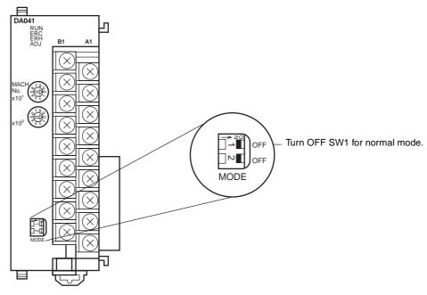
2. Set the unit number switch. Refer to 5-3-2 *Unit Number Switch* for further details.
