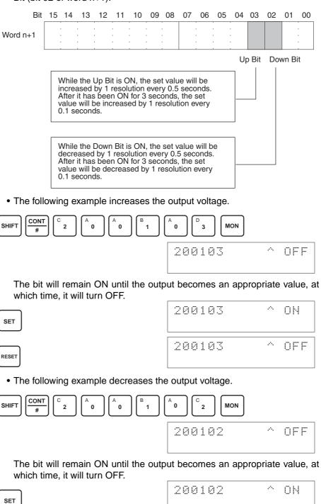
5. Check the 0-V/1-V/4 mA output, and then turn bit 04 (the Set Bit) of CIO word n+1 ON and then OFF again.
