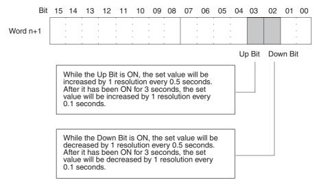
The following example increases the output voltage.
