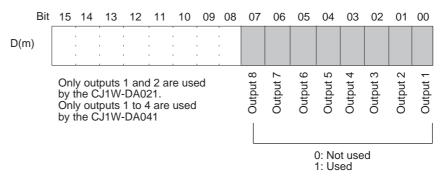
The analog output conversion cycle can be shortened by setting any unused output numbers to 0.
