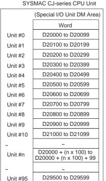
(Fixed Data Area) Input conversion permission loop D(m) mode setting Input signal range D(m+1)Data is automatically transferred to each unit D(m+2 to number when the power Sets number of m+9) is turned ON, or when samplings for mean (See note the Special I/O Unit value processing Ì.) Restart Bit is turned ON. Conversion time/ D(m+18)resolution and (See note 4.) operation mode m = 20000 + (unit number x 100)
