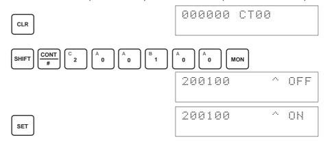
The analog input's digital conversion values while the Offset Bit is ON will be monitored in CIO word n+8.
