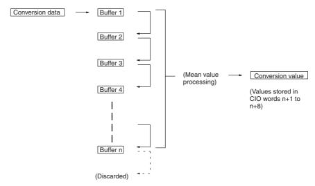
When "n" number of history buffers are being used, the first conversion data will be stored for all "n" number of history buffers immediately data conversion has begun or after a disconnection is restored.
