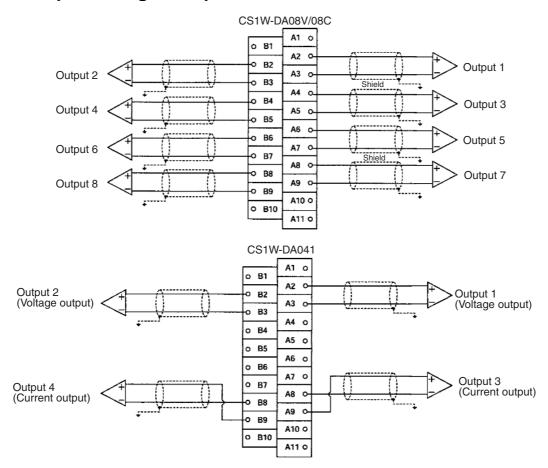
**Note** Crimp-type terminals must be used for terminal connections, and the screws must be tightened securely. Use M3 screws and tighten them to a torque of 0.5 N·m.
