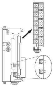
2. Mount and wire the Analog I/O Unit. Refer to 1-2-1 Mounting Procedure, 7-4 Wiring or 7-4-4 I/O Wiring Example for further details.
