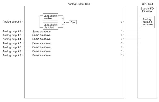
Note There are only four analog outputs for the CS1W-DA041.
