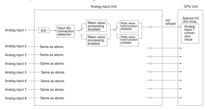
**Note** There are only four analog inputs for the CJ1W-AD041-V1.
