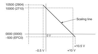
The following table shows the correspondence between input signals and converted scaling values. (The values shown in parentheses are binary data.)
