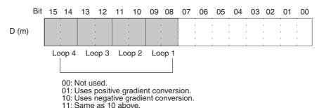
The response time of ratio conversion (input-to-output conversion) is 0.7 ms. For the DM word addresses,  $m = 20000 + (unit number \times 100)$ .
