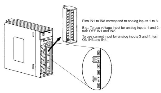
3. Mount and wire the Analog Input Unit. Refer to 1-2-1 Mounting Procedure, 2-4 Wiring or 2-4-4 Input Wiring Example for further details.
