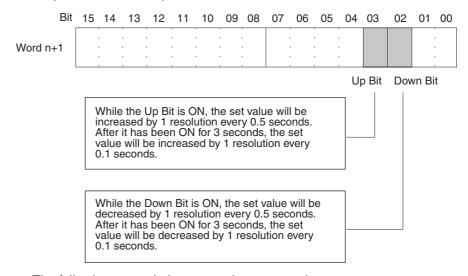
• The following example increases the output voltage.
