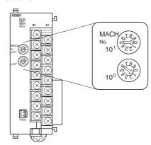
If the unit number is set to 1, words will be allocated to the Analog Input Unit in Special I/O Unit Area CIO 2010 to CIO 2019 and in the Special I/O Unit Area D20100 to D20199.
