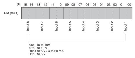
Note There are only four inputs for the CS1W-AD041(-V1).
