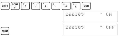
Caution Do not turn OFF the power supply or restart the Unit while the Set Bit is ON (data is being written to the EEPROM). Otherwise, illegal data may be written in the Unit's EEPROM and "EEPROM Errors" may occur when the power supply is turned ON or when the Unit is restarted, causing a malfunction.
