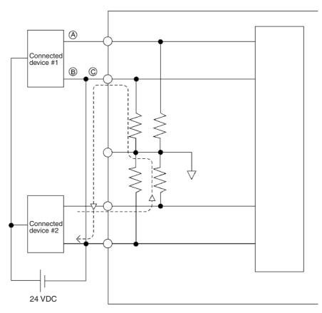
**Note** If the connected device #2 in the above example outputs 5 V and the power supply is shared by 2 channels as shown in the above diagram, approximately one third of the voltage, or 1.6 V, will be input at input 1.
