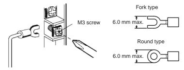
Connecting shielded cable to the Unit's AG terminals (A8, B8) can improve noise resistance.
