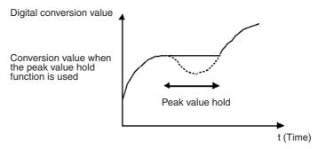
The peak value hold function can be set individually for each input number by turning on the respective bits (04 to 07) in CIO word n.
