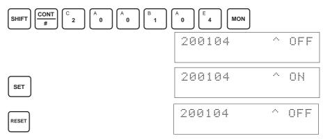
While the Clear Bit is ON, the adjusted value will be cleared and reset to the default offset and gain values when the Set Bit turns ON.
