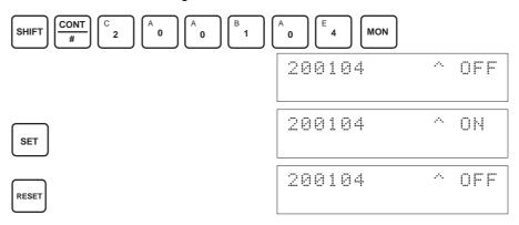
While the Offset Bit is ON, the offset value will be saved to the Unit's EE-PROM when the Set Bit turns ON.
