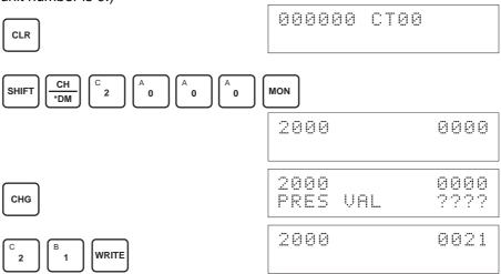
**Bits Used for Adjusting** Offset and Gain
