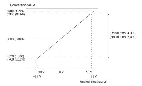
**Note** The conversion values for a range of –10 to 10 V will be as follows (for a resolution of 4,000):
