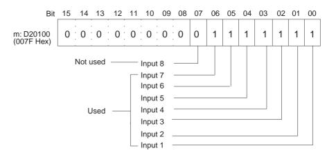
• The following diagram shows the input range settings. Refer to *DM Allocation Contents* on page 35 and 2-6-1 Input Settings and Conversion Values for more details.
