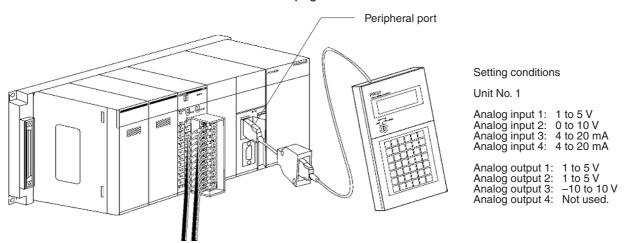
• The following diagram shows the input and output settings used. Refer to 6-6-1 Input Settings and Conversion Values or 6-7-1 Output Settings and Conversions for more details.
