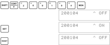
While the Gain Bit is ON, the gain value will be saved to the Unit's EE-PROM when the Set Bit turns ON.
