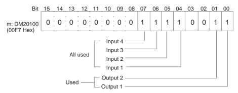
• The following diagram shows the input and output range settings. Refer to 7-6-1 Input Settings and Conversion Values or 7-7-1 Output Settings and Conversions for more details.
