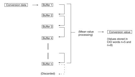
When "n" number of history buffers are being used, the first conversion data will be stored for all "n" number of history buffers immediately after data conversion has begun or after a disconnection is restored.
