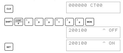
2. Check whether the output devices are connected.
