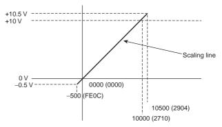
The following table shows the correspondence between output signals and converted scaling values. (The values shown in parentheses are 16-bit binary data.)
