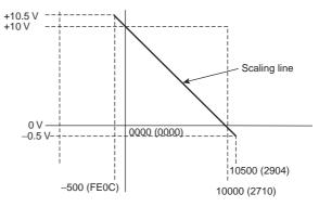
The following table shows the correspondence between output signals and converted scaling values. (The values shown in parentheses are 16-bit binary data.)
