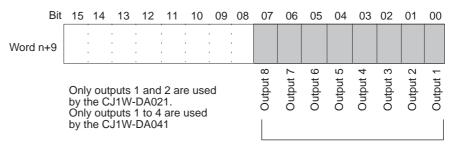
When a setting error is detected for a particular output, the corresponding bit turns ON. When the error is cleared, the bit turns OFF.
