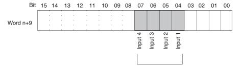
The respective bit turns ON when a disconnection is detected for a given input. When the disconnection is restored, the bit turns OFF.
