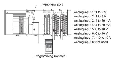
• The following diagram shows the input settings used. Refer to *DM Allocation Contents* on page 85 and 3-6-1 Input Settings and Conversion Values for more details.
