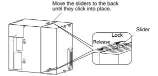
3. Attach an End Cover to the Unit on the right end of the Rack.
