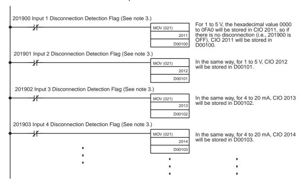
3. The input Disconnection Detection Flag is allocated to bits 00 to 07 of word (n + 9). Refer to *Allocations for Normal Mode* on page 39 for further details.
