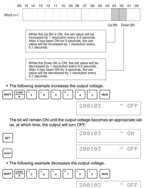
The bit will remain ON until the output voltage becomes an appropriate value, at which time, the output will turn OFF.
