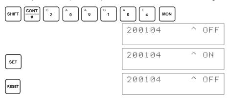
While the Gain Bit is ON, the gain value will be saved to the Unit's EE-PROM when the Set Bit turns ON.
