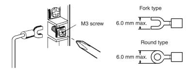
Connecting shielded cable to the Unit's AG terminals can improve noise resistance.
