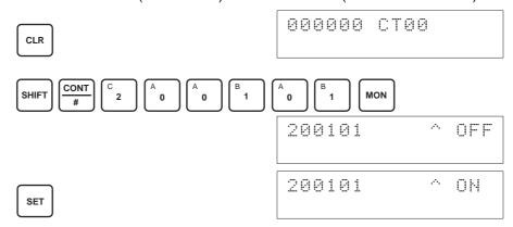
2. Check whether the output devices are connected.
