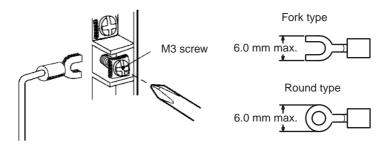
Connecting shielded cable to the Unit's AG terminals (A7, B7) can improve noise resistance.
