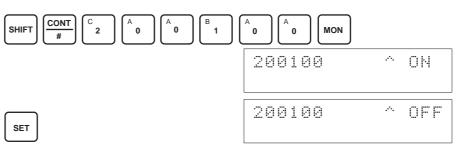
/!\ Caution Do not turn OFF the power supply or restart the Unit while the Set Bit is ON (data is being written to the EEPROM). Otherwise, illegal data may be written in the Unit's EEPROM and "EEPROM Errors" may occur when the power supply is turned ON or when the Unit is restarted, causing a malfunction.
