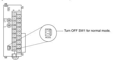
2. Set the voltage/current switch. Refer to 3-3-4 Voltage/Current Switch for further details.
