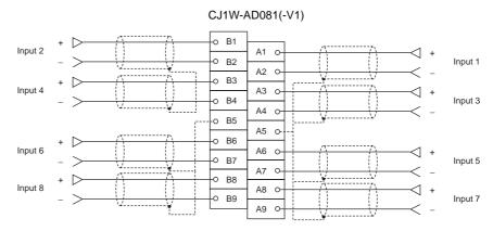
Note There are only four inputs for the CJ1W-AD041-V1. Inputs 5 to 8 are not used.
