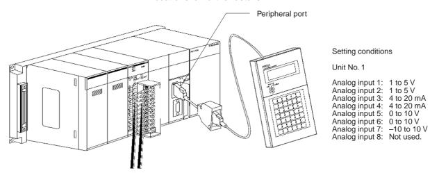
• The following diagram shows the input settings used. Refer to *DM Allocation Contents* on page 35 and 2-6-1 Input Settings and Conversion Values for more details.
