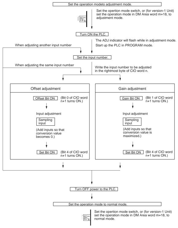
**Caution** Be sure to turn OFF the power to the PLC before changing the setting of the operation mode switch.
