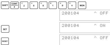
While the Clear Bit is ON, the adjusted value will be cleared and reset to the default offset and gain values when the Set Bit turns ON.
