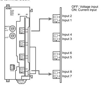
**Note** There are only four inputs for the CJ1W-AD041-V1.
