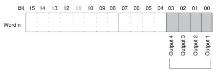
Analog conversion is executed while these bits are ON. When the bits are turned OFF, the conversion is stopped and the output data is held.
